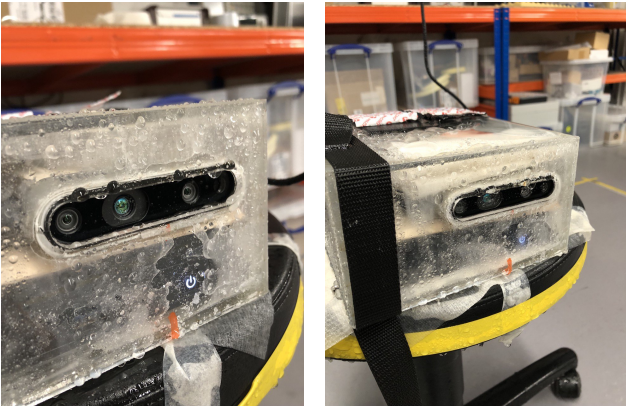
Fig. 1: The water-resistant box that hosts the processing unit and the depth camera. Right hand side shows stool mounting for moving conditions (Sec.V).
