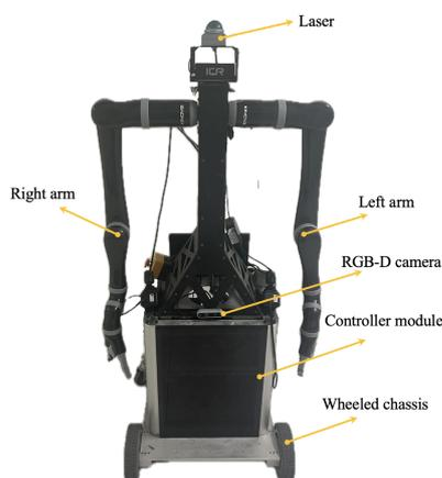
Fig. 2. Overview of the dual-arm mobile companion robot
