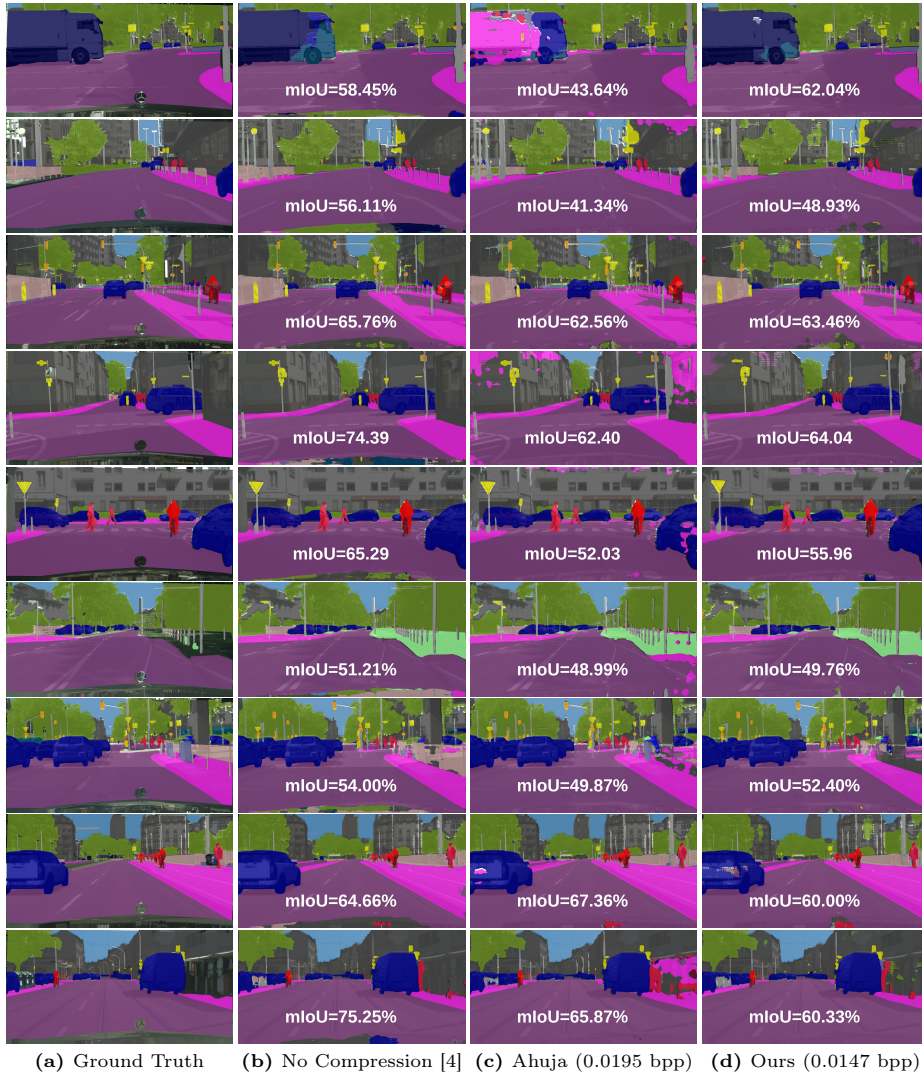
Fig. 13: Qualitative comparison of the proposed JD approach (" Ours ") against Ahuja et al. [1] on the Cityscapes dataset at low bitrates.
