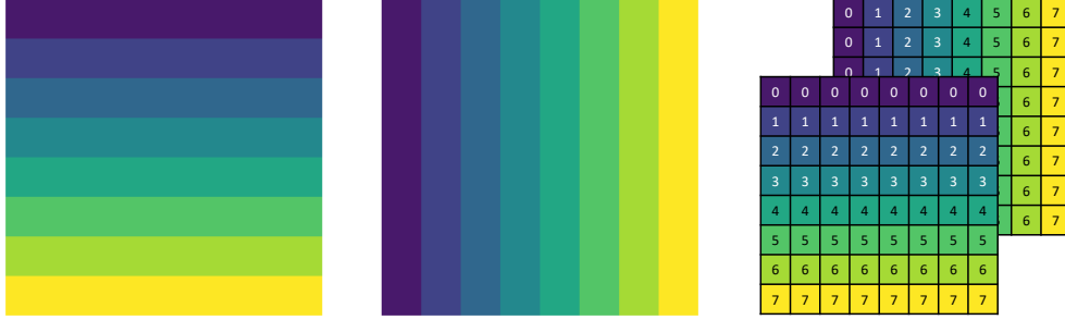
Figure S1: Mesh grids of input image. The intensity of pixels represents the coordinates in the two dimensions.
