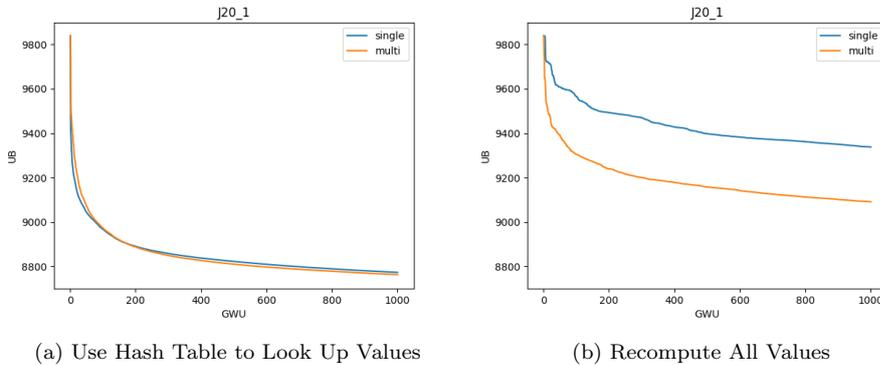
Fig. 4: Evolution of upper bound for externally-sampled instance of J20\_1 instance with  $N = 100$
