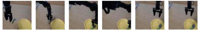
(b) Qualitative behavior of policy finetuned only both dense and sparse rewards: Robot lowers and place spatula on the plate and subsequently hovers above the placement position.
