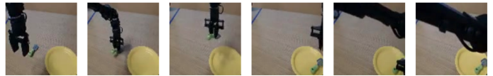
(a) Qualitative behavior of policy finetuned only on sparse rewards: Robot drops spatula on the plate from a height and continues moving rightward.
