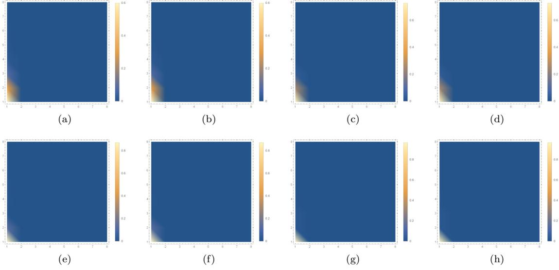
FIG. S2. (a)-(h) Density of all 8 wave functions of the system for  $L = 8$ ,  $t_x = \gamma_x = 1$ ,  $t_y = 2$ ,  $\gamma_y = \frac{3}{2}$ ,  $t_1 = \frac{1}{2}$ ,  $t_2 = \frac{5}{4}$ ,  $t_3 = t_4 = 0$ , which are all localized at  $x = 1$ .
