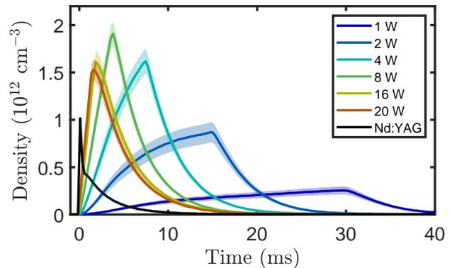
Figure 2. Time traces of atomic emission. Laser pulse energy is fixed at 30 mJ. The black trace shows Nd:YAG ablation yield, while other traces show laser heating at various powers. Filled area shows  $\pm 2\sigma_p$ , where  $\sigma_p$  is the standard error of the mean density at a given time.
