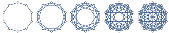
FIG. 1. Schematic representation of O(2) networks associated with circulant graphs of order N = 10 and increasing connectance from left to right, interpolating between the cycle graph C_N and the complete graph K_N .
