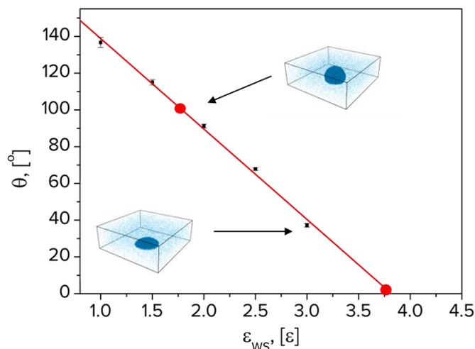
**Figure S10:** Dependence of contact angle of a water droplet as a function of the interaction energy  $\epsilon_{W-sub}$  between water and substrate obtained in the computer simulation. For  $\epsilon_{W-sub}$  values of  $1.7\epsilon$  and  $3.8\epsilon$  were chosen to obtain the intrinsic contact angles of the pure water at hydrophobic and hydrophilic substrates, respectively.
