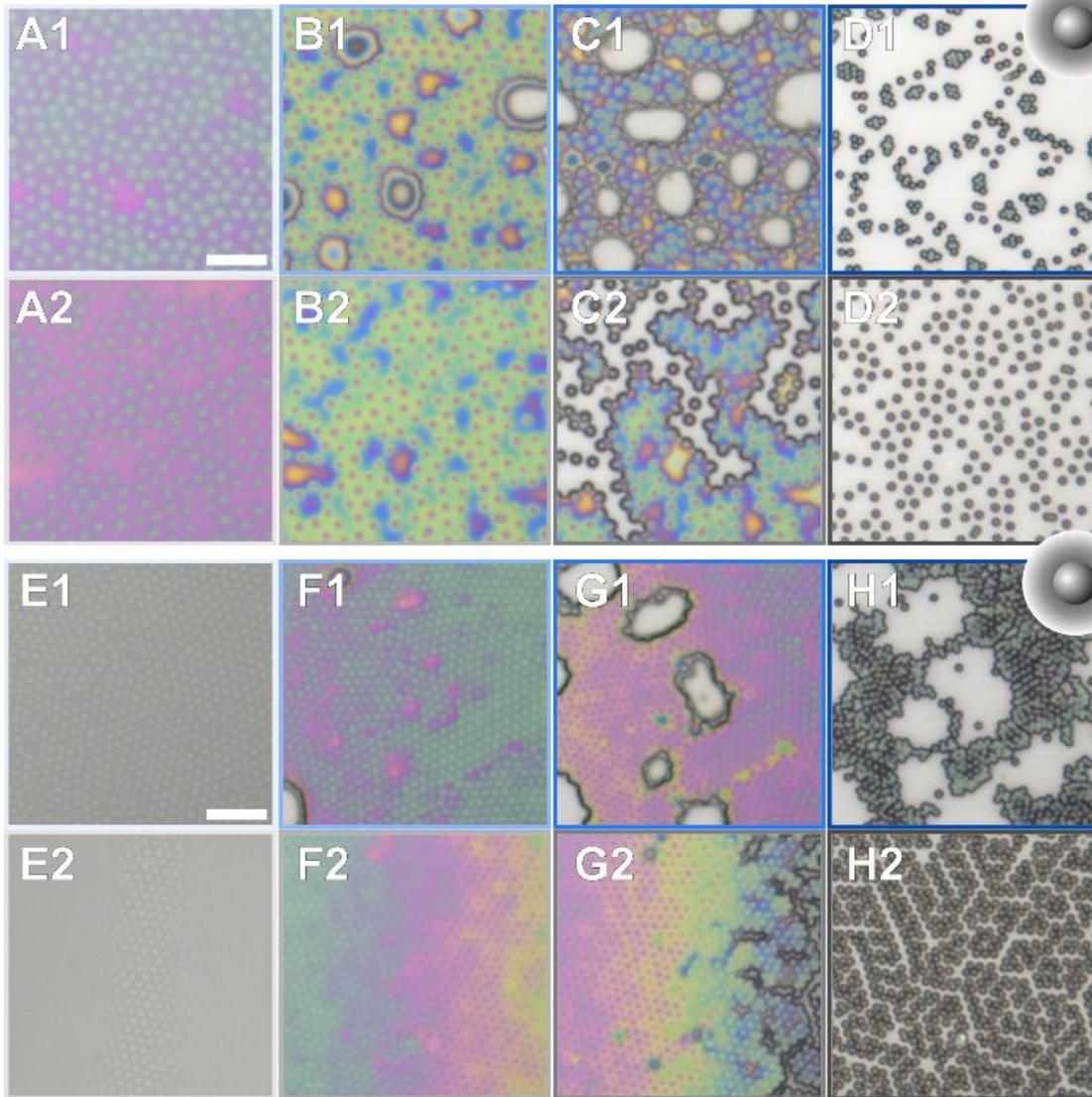
**Figure S4.** *In situ* monitoring of the drying of CS-medium film, transferred from  $\Pi$  near 10 mN/m, drying on hydrophilic (**A1-D1**) and on hydrophobic substrates (**A2-D2**). (**E1-H2**) are the same data sets for the microgel film transferred from  $\Pi$  near 30 mN/m. The scale bars correspond to 5  $\mu\text{m}$ .
