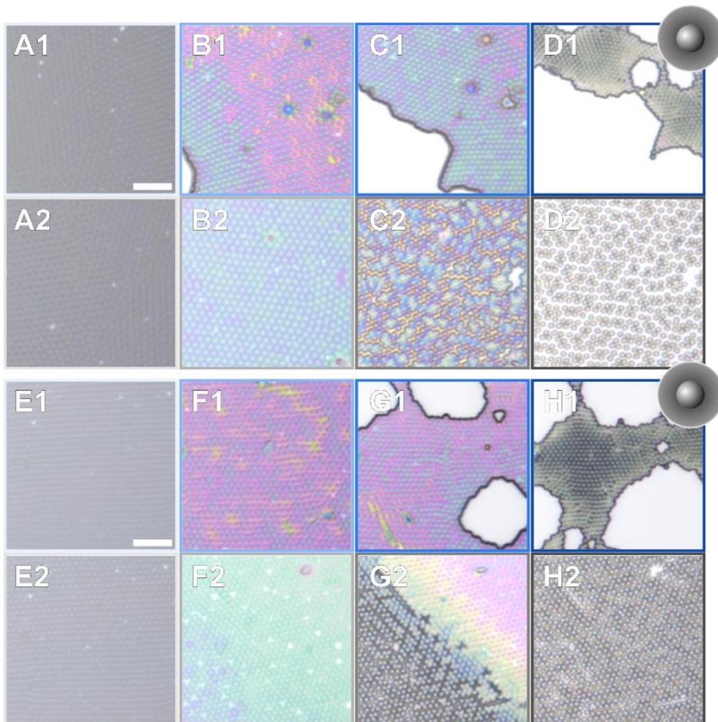
**Figure S16.** *In-situ* monitoring of the monolayer of CS-high transferred from  $\Pi$  near 10 mN/m, drying on hydrophilic (A1-D1) and on hydrophobic substrates (A2-D2). (E1-H2) are the same sets of data for the monolayer transferred from  $\Pi$  near 30 mN/m. The scale bars correspond to 5  $\mu\text{m}$ .
