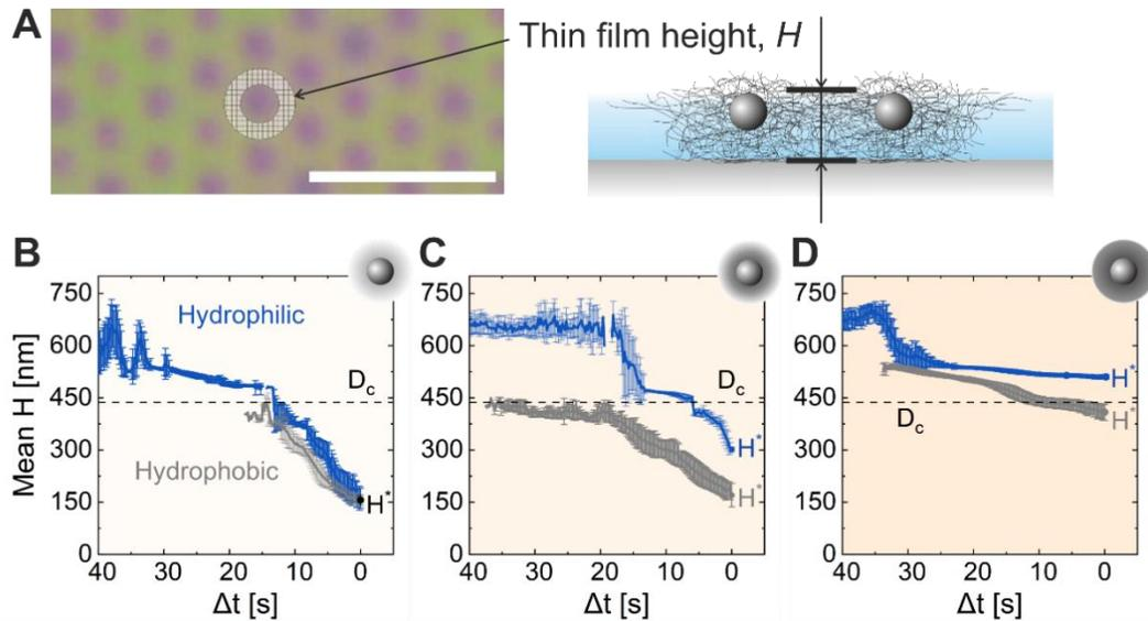
**Figure 8.** Film height,  $H$ , shown in an exemplary frame (A, left) and in a sketch (A, right). The scale bar corresponds to  $5 \mu\text{m}$ . Evolution of the height profiles of ten randomly chosen CS microgels in corresponding films drying on the hydrophilic (blue) and hydrophobic (grey) substrates for CS-low (B), CS-medium (C), and CS-high (D).
