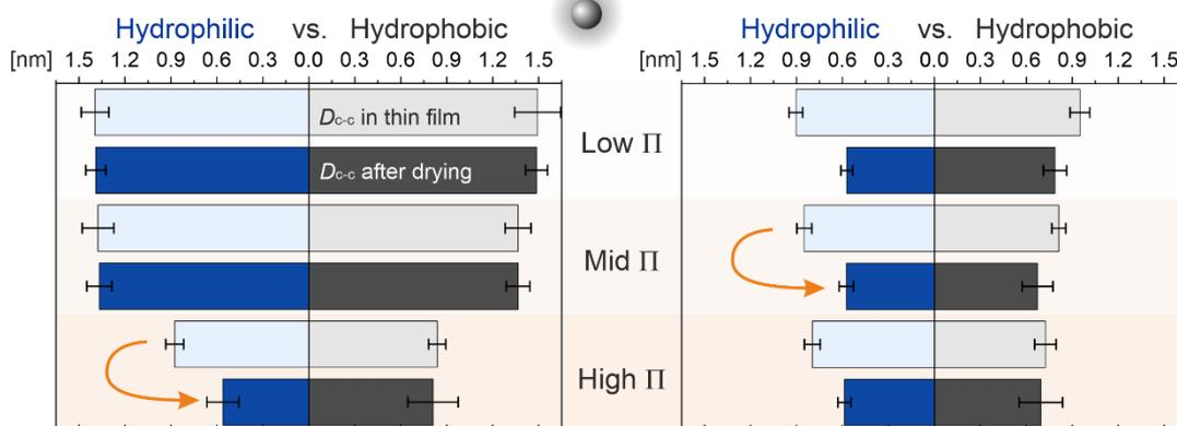
**Figure S17.** Center-to-center distance,  $D_{c-c}$ , of CS-low and CS-high. Films drying on hydrophilic (blue) and hydrophobic substrates (gray) in the thin fluid film (lighter color), as compared to that of dried monolayer (darker color).
