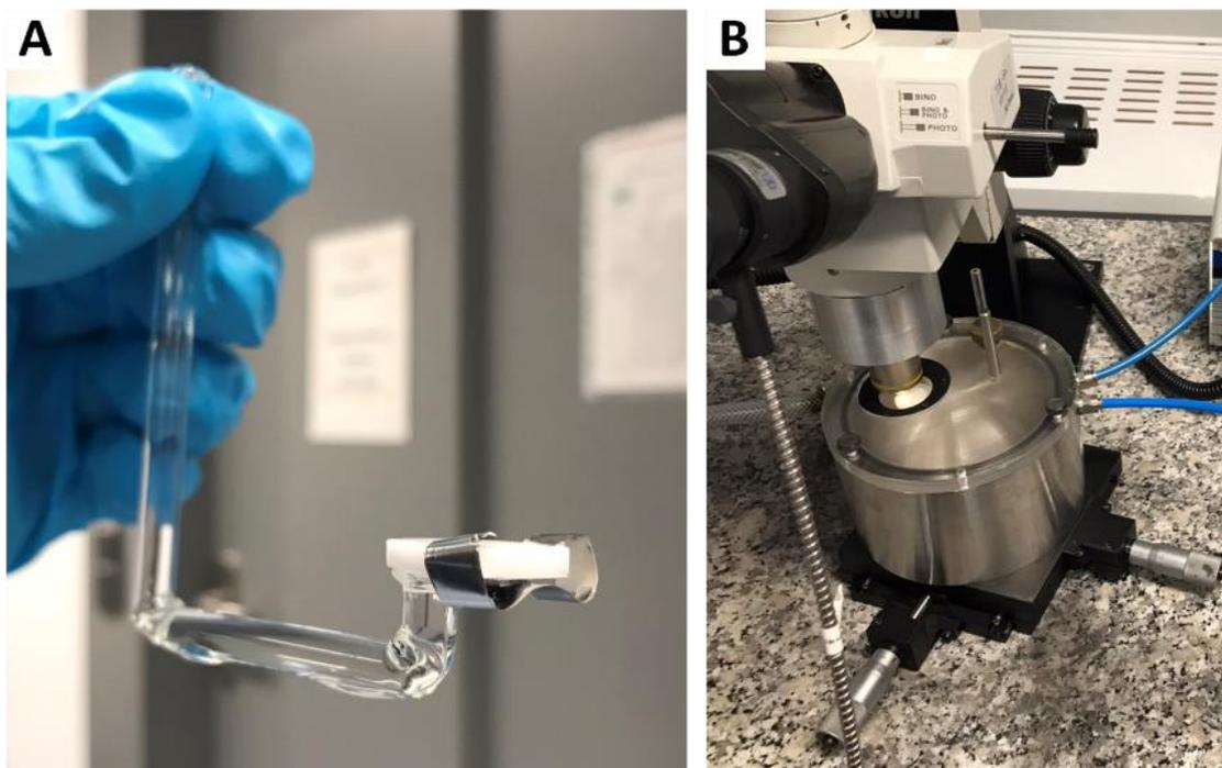
**Figure S6.** A) A porous glass plate is attached to a glass capillary tube (film holder) used for the thin film pressure balance technique. The sample is attached to the porous glass plate using a stainless-steel clamp. B) The stainless-steel pressure chamber with a quartz glass window is placed under a reflective light microscope.
