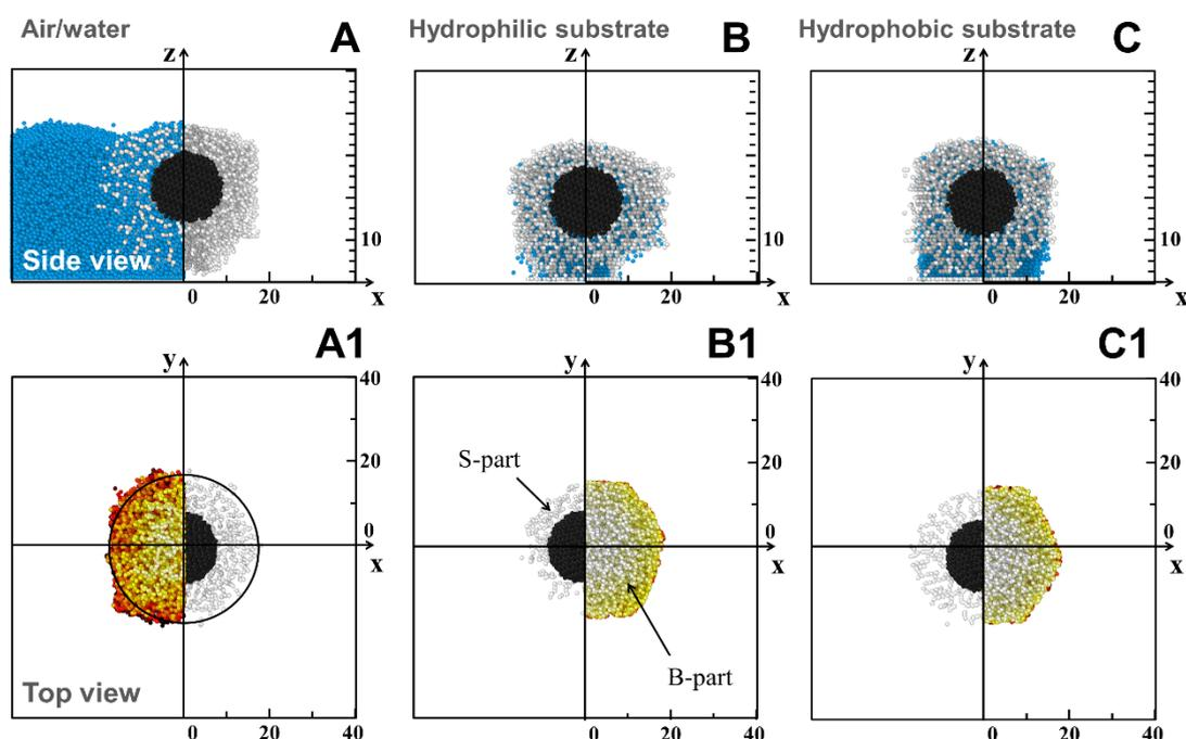
**Figure S14.** Illustration of the allocated microgel structure in the monolayer before (A-A1) and after drying in the case of hydrophilic (B-B1) and hydrophobic (A2-E2) substrates. The monolayer was transferred at a high compression degree. (A1-C1) Height map / Contact area at the interface. All snapshots are obtained using the Open Visualization Tool (OVITO) [13].
