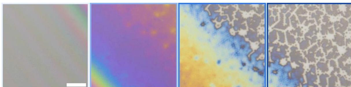
**Figure S20.** Drying of a small CS microgel ( $D_c$ : 105 nm  $D_h$ : 504 nm, cross-linker density: 5 mol.%) film on a hydrophilic substrate, transferred from  $\Pi$  approx. 30 mN/m, scale bar corresponds to 5  $\mu\text{m}$ .
