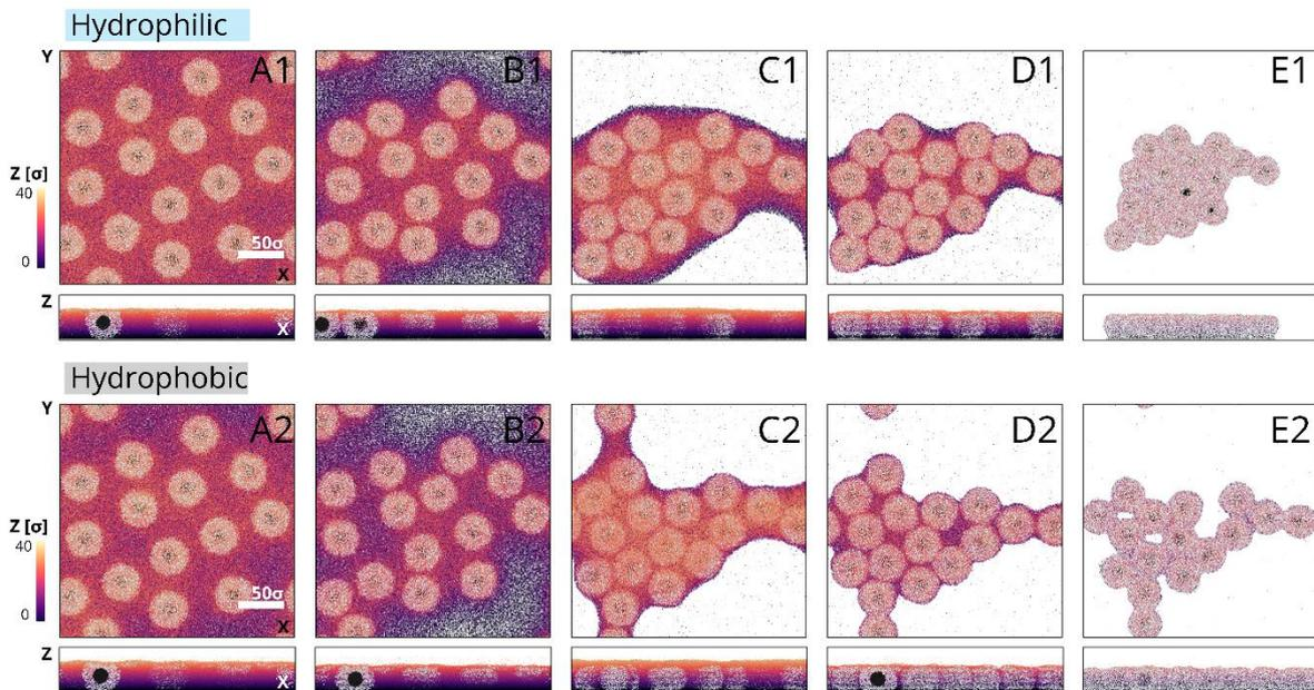
**Figure 5.** Illustration (top views) of the different stages of microgel film obtained at low  $\Pi$  drying on hydrophilic (A1-E1) and hydrophobic (A2-E2) substrates as revealed by computer simulations. The narrow panels below the top views are the corresponding side views, i.e.,
