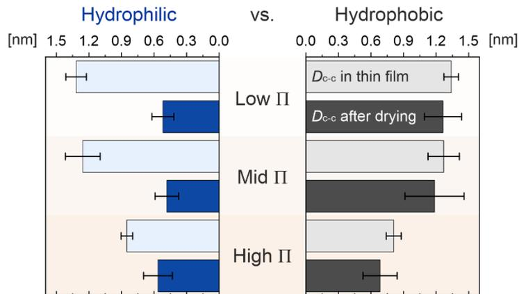
**Figure S5.** Center-to-center distance,  $D_{c-c}$ , of CS-medium film drying onto hydrophilic (blue) and hydrophobic (gray) substrates. Distances in thin film are shown using lighter colors and compared to the ones of fully dried microgel clusters (darker colors). The error bars are the standard deviations of the first peaks of the radial distribution functions.
