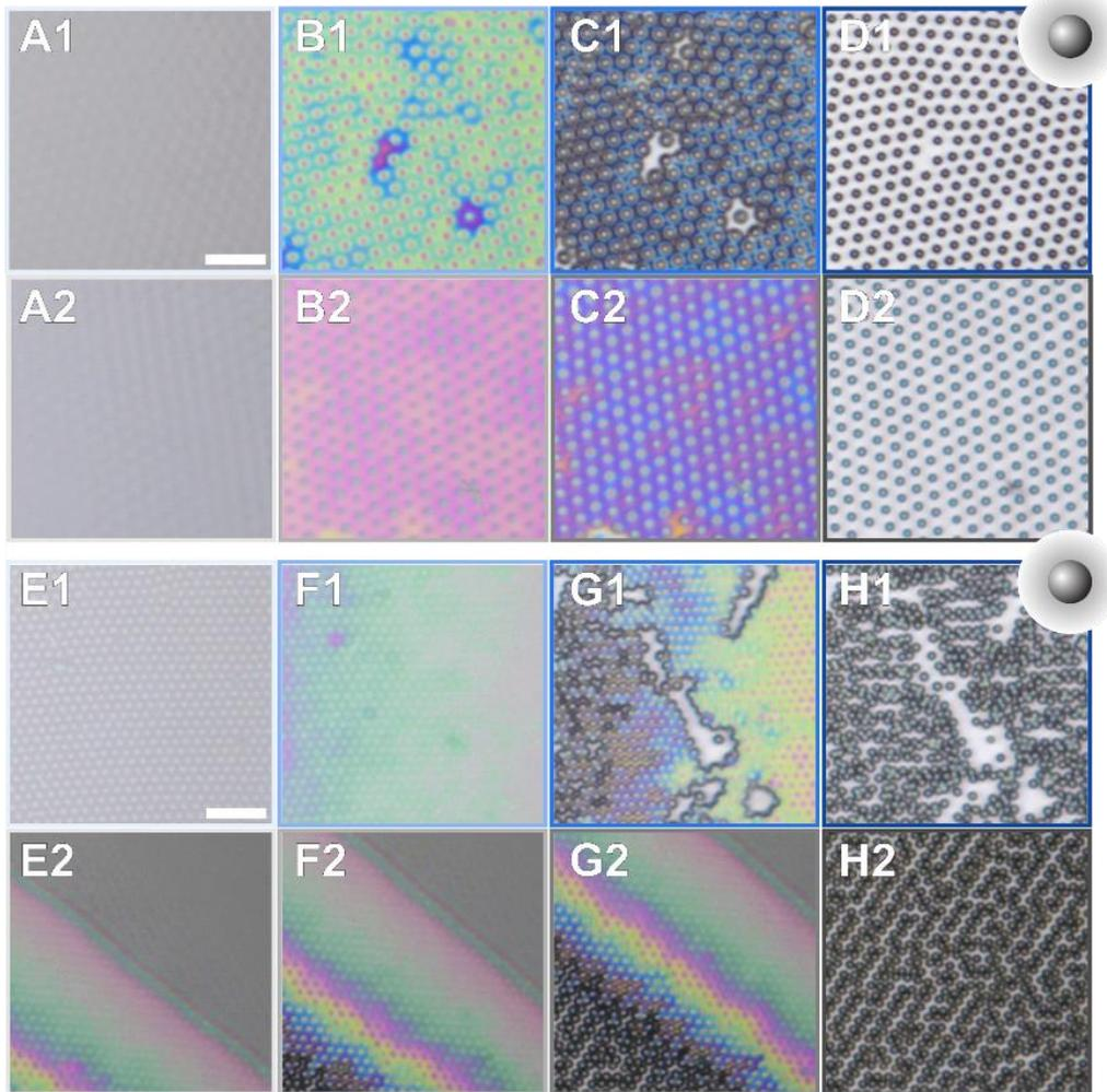
**Figure S15.** *In-situ* monitoring of the monolayer of CS-low transferred from  $\Pi$  near 10 mN/m, drying on hydrophilic (A1-D1) and on hydrophobic substrates (A2-D2). (E1-H2) are the same sets of data for the monolayer transferred from  $\Pi$  near 30 mN/m. The scale bars correspond to 5  $\mu\text{m}$ .
