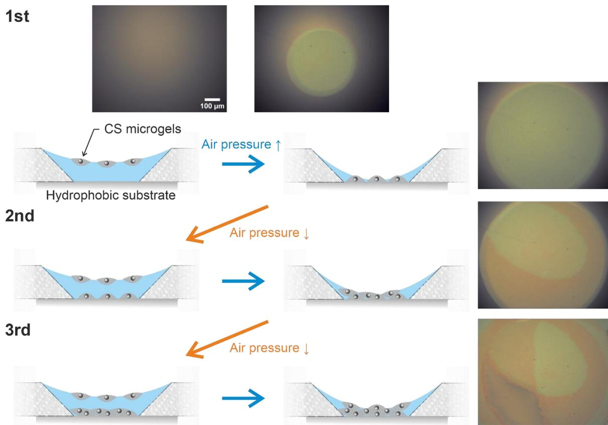
**Figure S7.** The interface oscillation experiment (3 cycles) using a modified thin film pressure balance setup, depicted in **Figure 3**, only results in the formation of multilayers (3 layers of CS-medium film, indicated by the different colors of the patches) when attempted on hydrophobic substrates.
