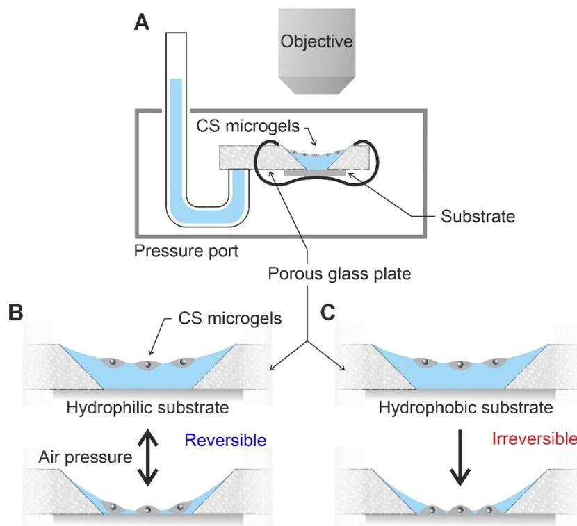
**Figure 3.** Schematic illustrations of a modified thin film pressure balance (TFPB) setup (A) and the microgel-laden interface oscillation experiment by pressure modulation using a hydrophilic substrate: far away from the solid substrate (B) and in the thin film on the substrate (C). Videos recorded for experiments on a film of CS-medium are provided in the SI.
