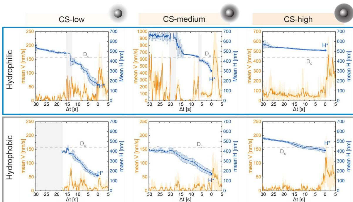
**Figure S21.** The mean velocity,  $V$ , and film height,  $H$ , of 10 randomly chosen CS microgels are plotted against normalized time, where 0 is the onset of the collapse of the individual microgels.  $D_c$  and  $H^*$  denote the diameter of the core and the critical height of the monolayer, respectively. The shadowed areas (grey) are frames where the monolayers were out-of-focus. Monolayer drift with preferred directions is baseline-subtracted.
