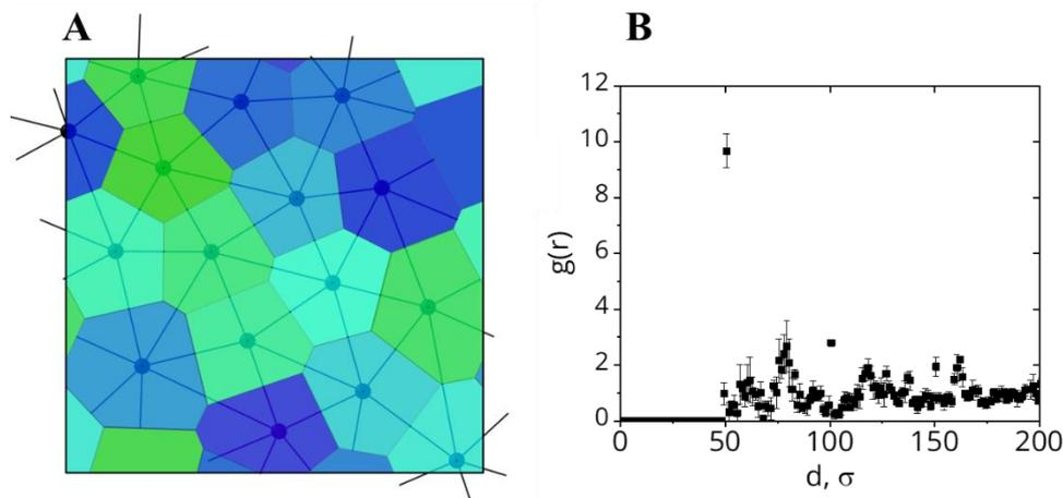
**Figure S11.** (A) 2D Voronoi tessellation of the simulation box, taking the center of mass of the solid core particles as Voronoi cell centers. (B) The radial pair distribution function, RDF, is for the center of mass of the solid core particles. Cases of low compression degree. Low surface affinity to microgels.
