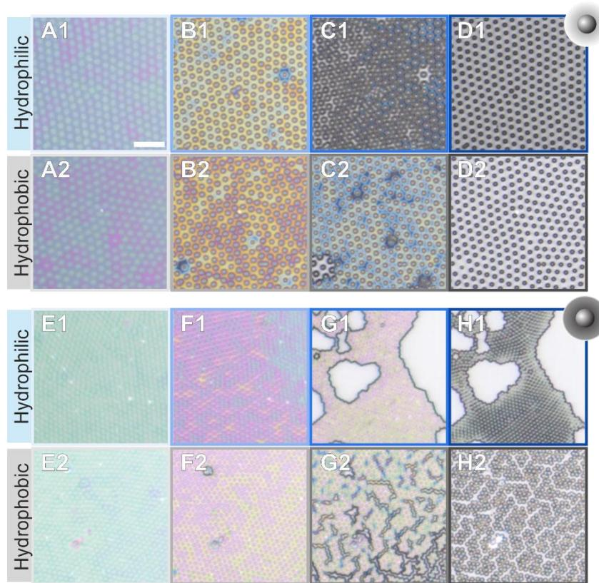
**Figure 6.** Reflected light microscopy images of CS-low (**A-D**) and CS-high microgel films (**E-H**) at mid  $\Pi$  ( $\sim 20$  mN/m) transferred onto hydrophilic (**A1-D1, E1-H1**) and hydrophobic substrates (**A2-D2, E2-H2**) during the drying process. The scale bar corresponds to  $5\mu\text{m}$ .
