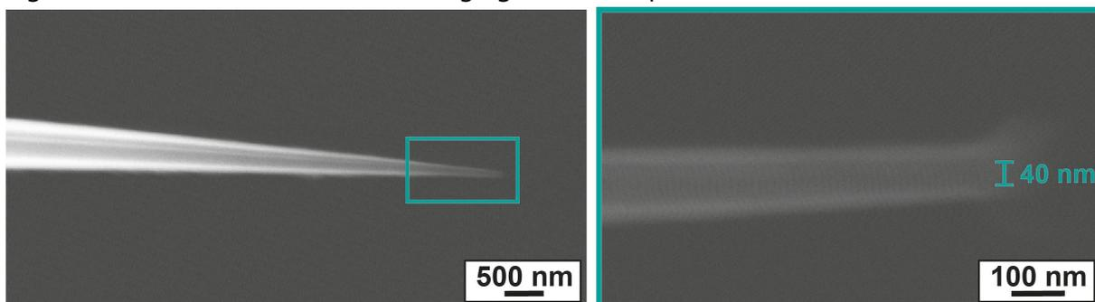
**Figure S1:** STEM-in-SEM image of the capillary probe tip.
