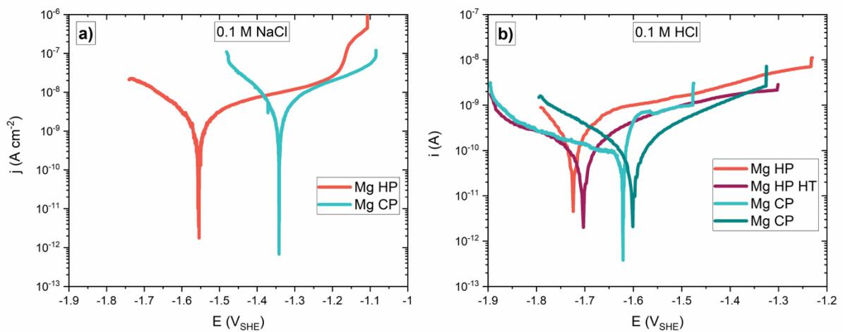
Figure 3: Potentiodynamic polarization curves performed on different pure Mg materials a) at a scan rate of 0.5 mV s<sup>-1</sup>, using the microcapillary technique with a 100 μm diameter microcapillary filled with 0.1 M NaCl and b) at a scan rate of 10 mV s<sup>-1</sup>, using the SEN technique with a 40 nm probe filled with 0.1 M HCl. Note that the current is corrected for the area in the case of the microcapillary technique (area: 0.8 mm<sup>2</sup>) but not for the SEN measurements.
