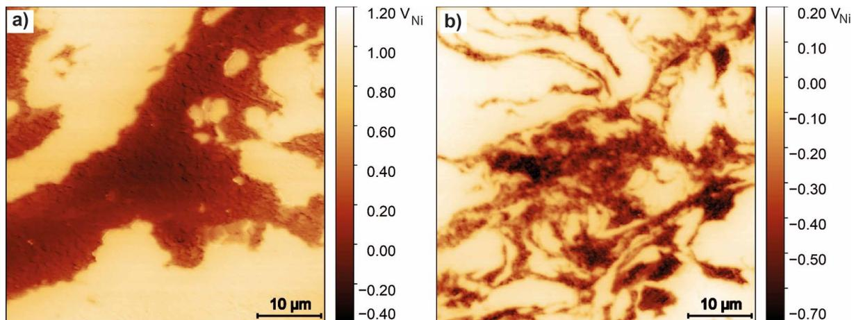
**Figure S14:** SKPFM based Volta potential measurements on sputtered a) coarse and b) nanostructured Mg50-Fe composite surfaces. Note that the Volta potentials are expressed versus a Ni reference sample.
