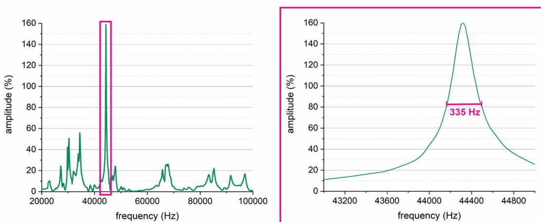
**Figure S2:** Typical example of the frequency-dependent response of the oscillating capillary probe. In this case, the probe resonance frequency is 44.320 kHz and its Q-factor is 130 %.
