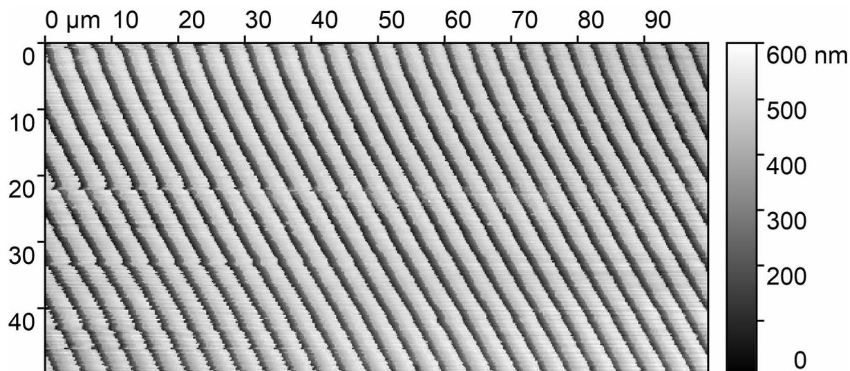
**Figure S3:** Mapping of TGZ03 calibration grid (3  $\mu\text{m}$  pitch, height: 496 nm, MikroMasch) with a 40 nm probe filled with MilliQ water. This shows the ability of the SEN setup to track even small topographic changes over long time (> 24 h acquisition time).
