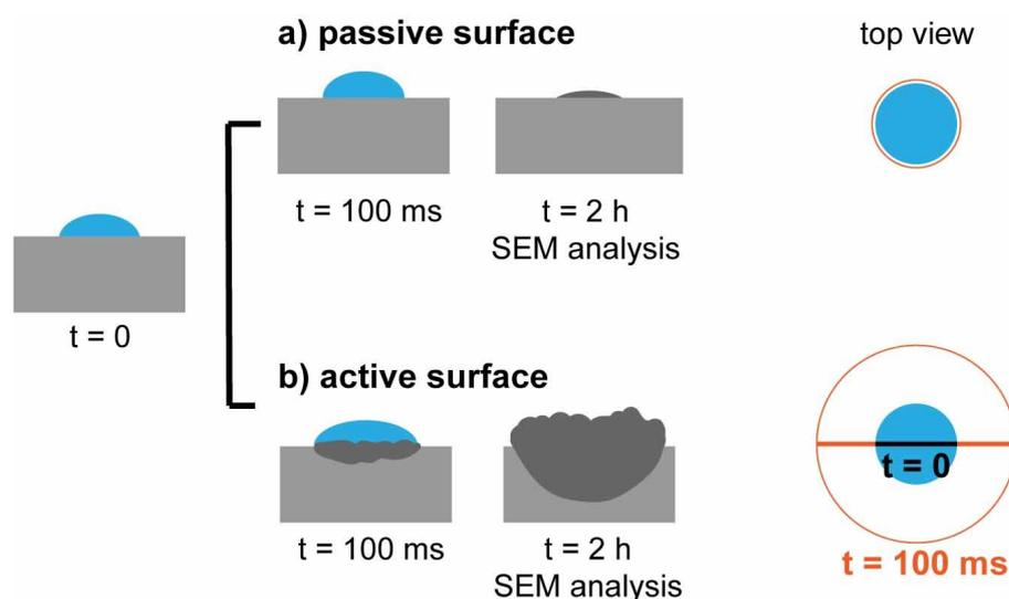
**Figure S5:** Schematics showing the evolution of the exposed area on a) passive and b) active surfaces. The effective surface is not expected to change on passive surfaces while on active surfaces, it is expected to drastically increase as soon as active dissolution starts, which can lead to an estimation mismatch. Therefore, the current was not corrected for the area in SEN-based measurements.
