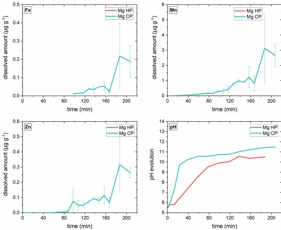
**Figure S9:** Dissolved amount of trace-elements during immersion of high purity (HP) and commercially pure (CP) Mg in unbuffered 0.1 M NaCl and the corresponding pH evolution.
