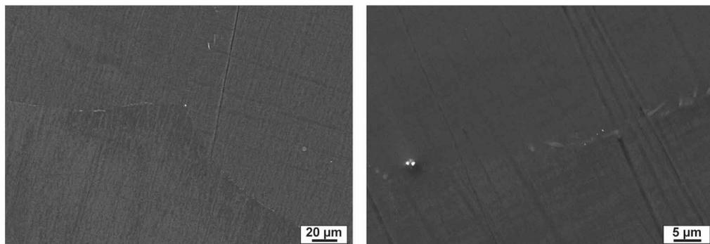
**Figure S6:** Microstructure of the pure Mg grades studied. a) commercially pure Mg (Mg CP); high purity Mg b) as-produced (Mg HP) and c) after heat-treatment for 24 h at 525 °C under Ar atmosphere (Mg HP HT).
