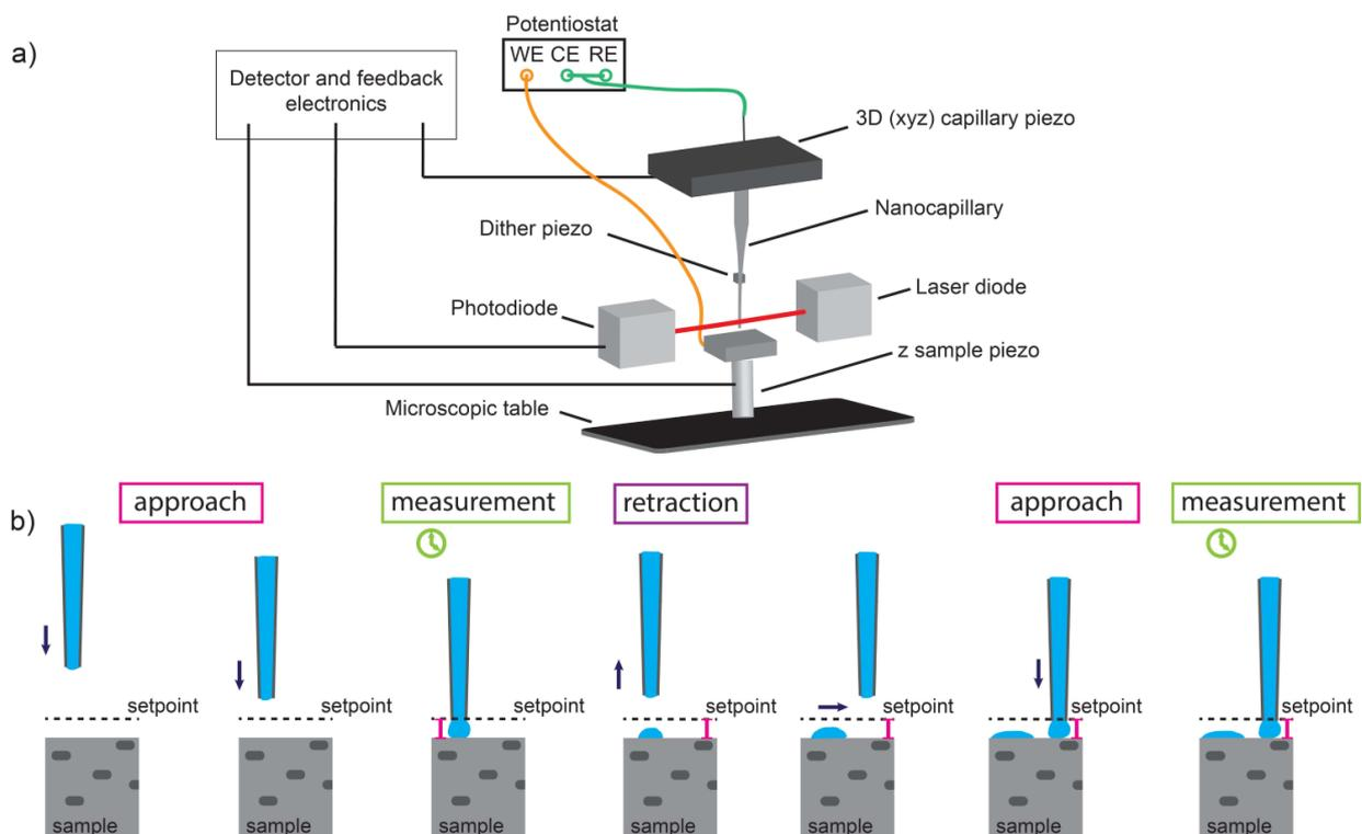
Figure 1: a) Schematic description of the scanning electrochemical nanocapillary (SEN) setup. b) details of the SEN intermittent contact principle on flat samples based on meniscus-confined electrochemical measurements. After the approach, the probe remains on a point for some time (from a few milliseconds to seconds) to allow electrochemical measurements. The probe is then retracted and moved to the next point.
