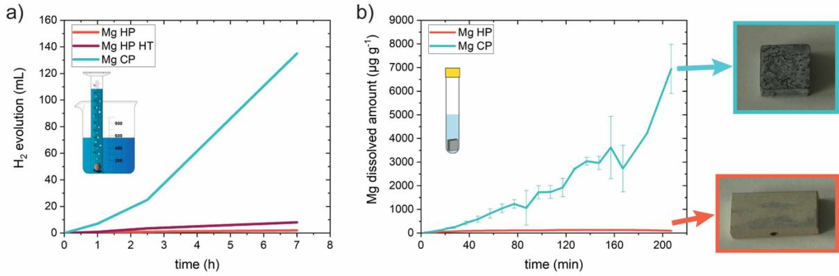
**Figure S8:** Effect of impurities on the corrosion rates of pure Mg. a) Hydrogen evolution and b) amount of dissolved Mg during immersion of high purity (HP, HP-HT) and commercially pure (CP) Mg alloys in unbuffered NaCl solutions.
