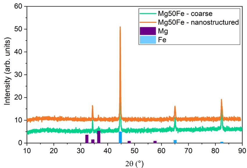
**Figure S13:** XRD scans for the two Mg50-Fe composites and corresponding peak positions for Mg (hcp, collection code: 29734) and Fe (bcc, collection code: 52258). These reference powder diffraction patterns were taken from the online ICSD database.
