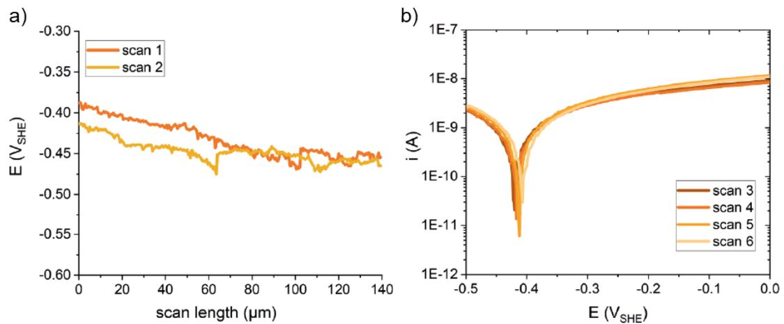
**Figure S10:** SEN measurements on Fe 99.5% with a 40 nm probe filled with 0.1 M HCl. a) potential scans with a measurement duration of 100 ms per point and b) potentiodynamic polarization curves at a scan rate of  $10 \text{ mV s}^{-1}$ . Note that the current is not corrected for the area.
