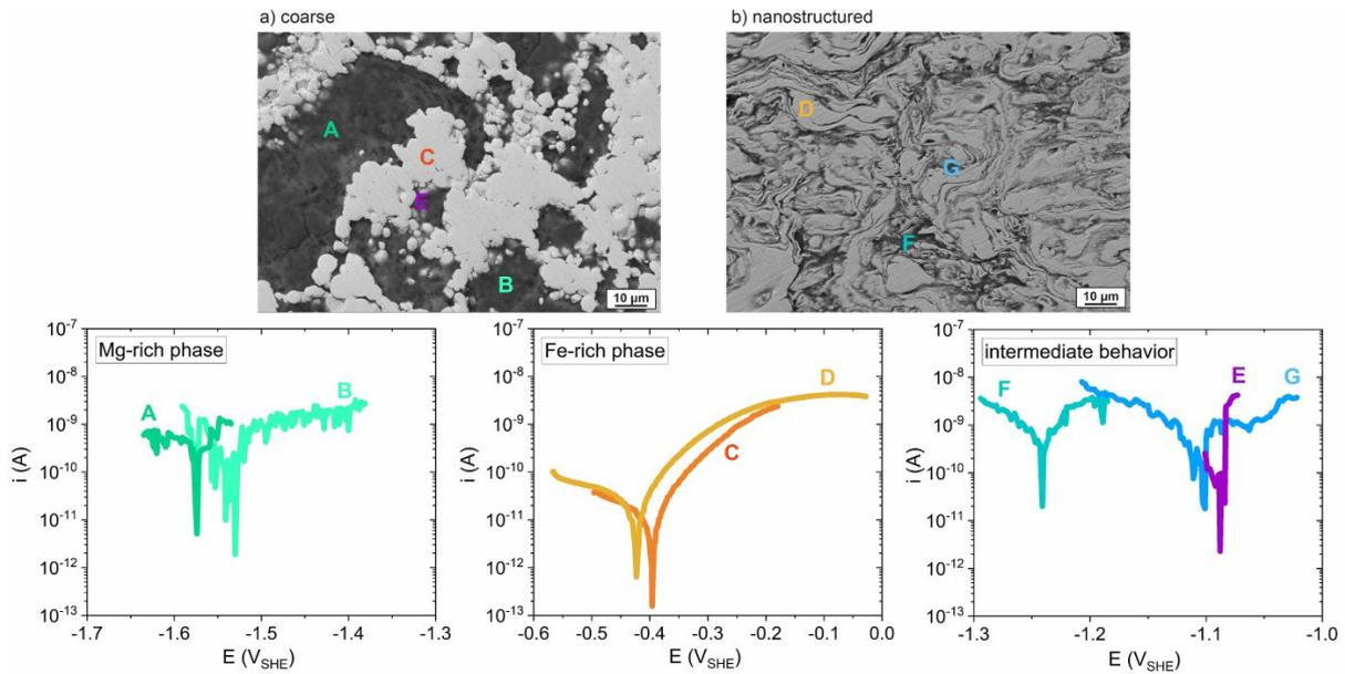
Figure 11: Typical SEN potentiodynamic polarization curves performed on two Mg50-Fe composites with a 40 nm probe filled with 0.1 M HCl at a scan rate of 10 mV s<sup>-1</sup>. Note that the current is not corrected for the area.
