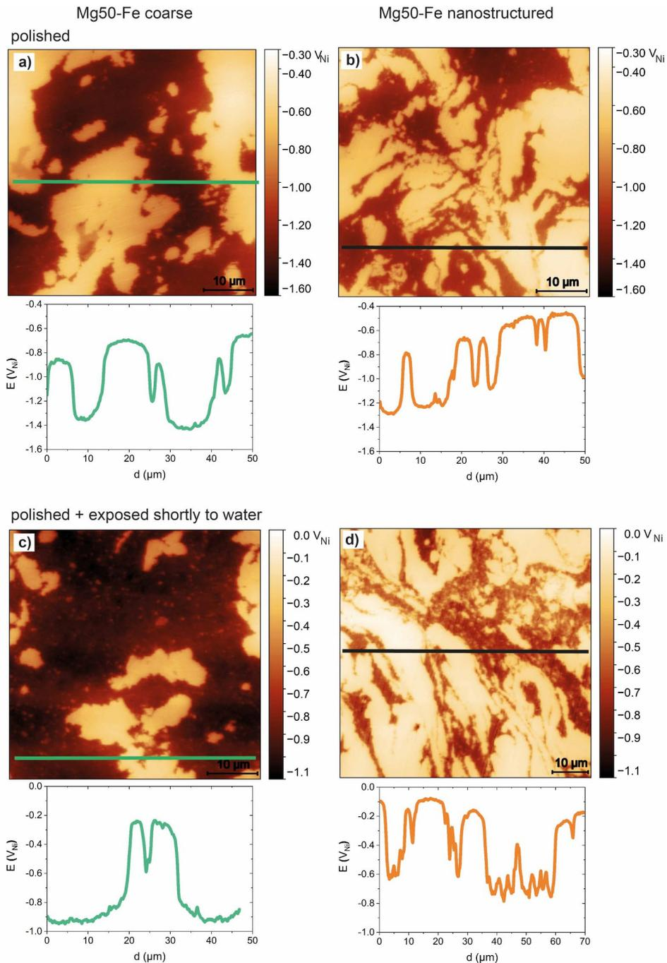
Figure 9: Volta potential measurements of polished a) coarse and b) nanostructured Mg50-Fe composites. c) and d) are the Volta potential measurements on the two composites after short exposure to water. Note that the Volta potentials are expressed versus a Ni reference sample.
