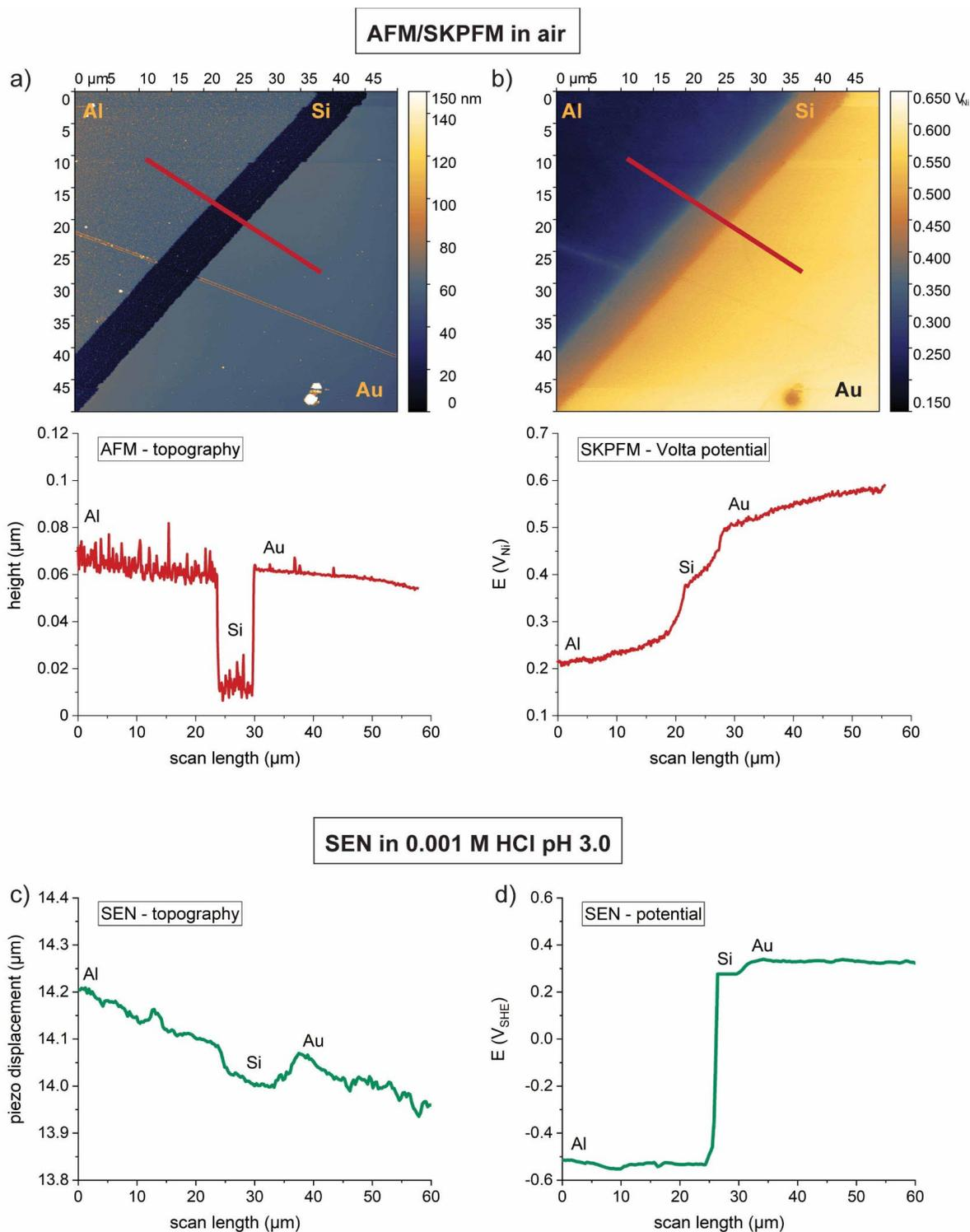
**Figure S4:** a) AFM and b) SKPFM imaging of the PFKPFM-SMPL reference sample in air. Note that the Volta potentials are expressed versus a Ni reference. Corresponding c) topographic and d) potential scans obtained by SEN measurements with a 40 nm probe filled with 0.001 M HCl at pH 3.0.
