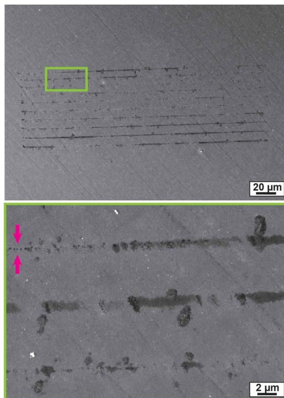
Figure 6: Secondary electron (SE) SEM image after SEN line scans on CP Mg surfaces, using a 40 nm probe filled with 0.1 M HCl. The SEN line scans were performed with a step size of 400 nm, a scanning rate of 500 nm s<sup>-1</sup> and a measurement time of 100 ms on each point. The distance between each line scan is 5 μm.
