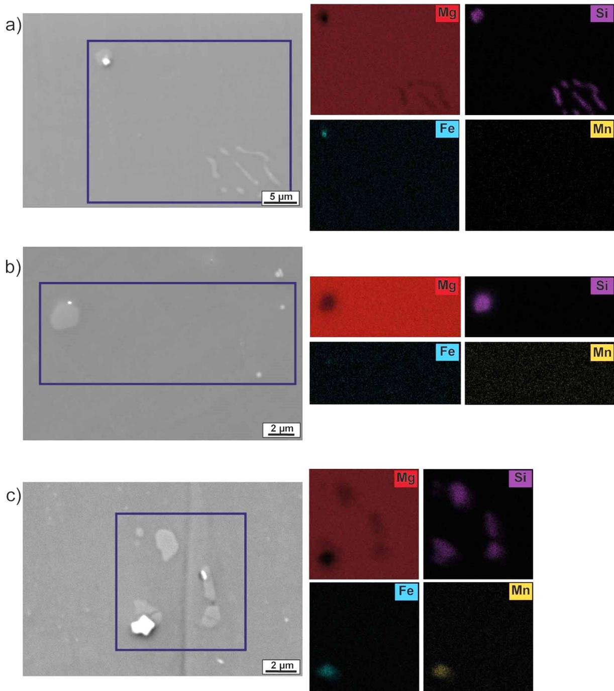
**Figure S7:** SEM images and corresponding energy-dispersive X-ray spectroscopy (EDX) maps of particles found in high purity Mg a) as-produced (HP) and b) after heat-treatment for 24 h at 525 °C under Ar atmosphere (HP HT) and c) in commercially pure Mg materials (CP)
