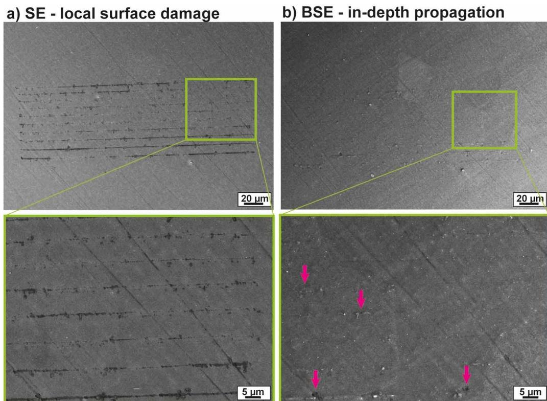
**Figure S11:** a) Secondary electron (SE) and b) Backscattered electron (BSE) images after SEN line scans on Mg CP surfaces, using a 40 nm probe filled with 0.1 M HCl. The SEN line scans were performed with a step size of 400 nm, a scanning rate of  $500 \text{ nm s}^{-1}$  and a measurement time of 100 ms on each point. The distance between each line scan is 5  $\mu\text{m}$ .
