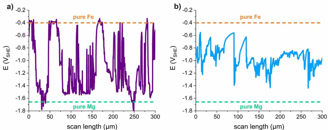
Figure 8: Typical SEN OCP scans for a) coarse and b) nanostructured Mg50-Fe composites, using a 40 nm probe filled with 0.1 M HCl. The SEN line scans were performed with a step size of 200 nm, a scanning rate of  $500 \text{ nm s}^{-1}$  and a measurement time of 100 ms on each point. The local potential changes displayed are obtained by averaging the potential values over the last 25 ms.
