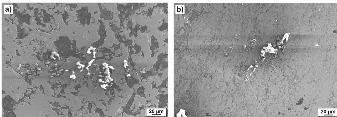
Figure 10: SE SEM image after SEN line scans on a) coarse and b) nanostructured Mg50-Fe composite surface, using a 40 nm probe filled with 0.1 M HCl. The SEN line scans were performed with a step size of 200 nm, a scanning rate of 500 nm s<sup>-1</sup> and a measurement time of 100 ms on each point.
