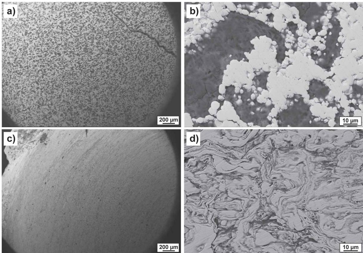
**Figure S12:** SEM images of Mg50-Fe composites produced by a) and b) cyclic HPT at room temperature (coarse) and c) and d) monotonic HPT at 300 °C (nanostructured).
