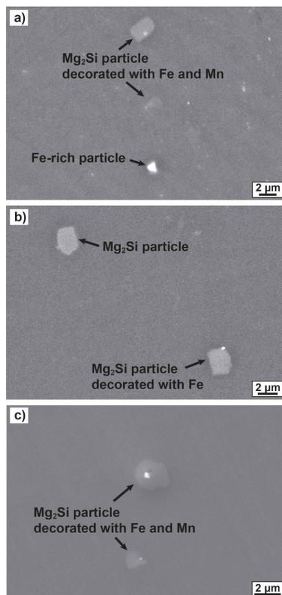
Figure 2: SEM images of particles found in a) commercially pure (CP) Mg specimens and high purity (HP) Mg specimens b) as-produced and c) after heat-treatment for 24 h at 525 °C (HP-HT).
