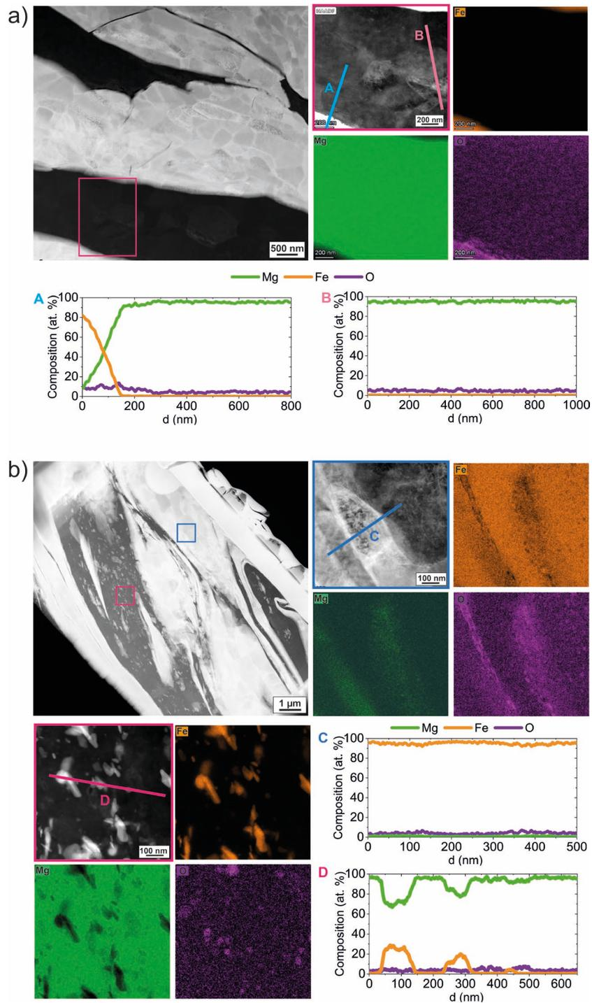
Figure 7: High-angle annular dark-field (HAADF)-STEM images and energy-dispersive X-ray spectroscopy (EDX) maps of a) coarse and b) nanostructured Mg50-Fe composites.
