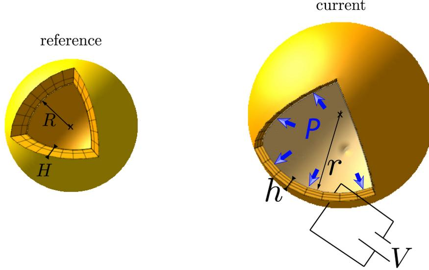
**Figure 1. Schematic view of the dielectric elastomer balloon in the reference and current configurations. Note that the thicknesses are amplified in the figure for illustration purposes. In the analysis, they are assumed to be infinitesimal compared to the radii, leading to the membrane approximation [50].**
