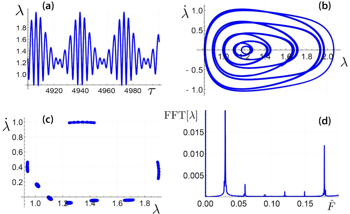
Figure 5. Quasiperiodic vibrations of a DE balloon made of early-stiffening material with  $N = 4$ , for  $\bar{P} = 0.8$ ,  $\bar{V}_{DC} = 0.3836$ ,  $\bar{V}_{AC}/\bar{V}_{DC} = 0.1$ . (a) Time-stretch diagram, (b) Phase portrait, (c) Poincaré section, (d) Fast Fourier Transform.
