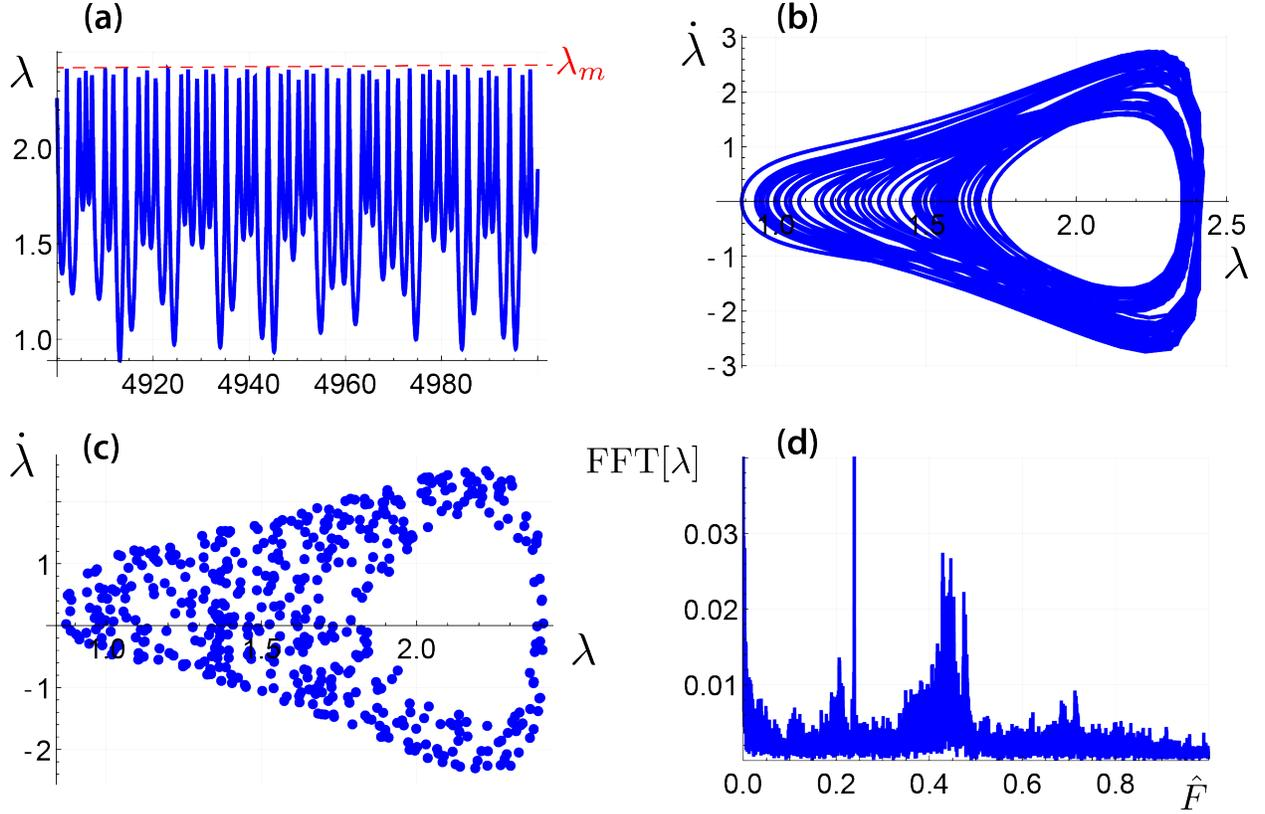
Figure 7. Chaotic vibrations of the DE balloon for  $\bar{P} = 0.8$ ,  $\bar{V}_{DC} = 0.7$ ,  $\frac{\bar{V}_{AC}}{\bar{V}_{DC}} = 0.1$  and  $N = 4$ . (a) Time-stretch diagram, (b) Phase portrait, (c) Poincaré section, (d) FFT.
