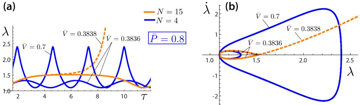
**Figure 4.** The DC dynamic response of the DE balloon for  $\bar{P} = 0.8$ , when the number of Kuhn segments is  $N = 4$  (early strain-stiffening effect) and  $N = 15$  (late strain-stiffening effect). In the latter case, as soon as the voltage exceeds the critical voltage threshold  $\bar{V}_{DC} = 0.3837$ , the motion loses its periodicity. In the former case, there is no critical voltage of dynamic instability, even though there is one for static instability.
