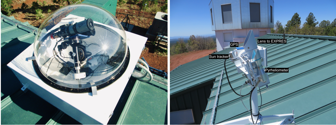
Figure 1. Left: The original design of the Lowell Observatory Solar Telescope (LOST). This telescope is a traditional equatorial mount that is housed in a weather-sealed enclosure. Right: The upgraded design of LOST features a dedicated solar tracker from EKO systems and a custom-designed weather-sealed lens assembly. Both telescopes were mounted on the roof of the auxiliary building at the Lowell Discovery Telescope site in Happy Jack, AZ, and fiber-fed into the EXtreme PREcision Spectrograph (EXPRES).
