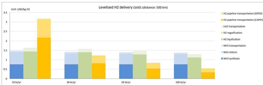
**Fig. 11.** Impacts of transport volume on hydrogen delivery cost
