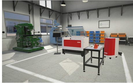
Figure 3: Laboratory with the Trotec Speedy 400 laser cutting machine and a working table
