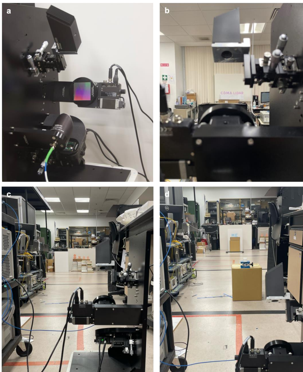
Fig. 19. Photos of the experimental setup: (a) Identity-enabled CDMA LiDAR prototype; setups for (b) 5 m scan, (c) 10 m scan, and (d) near-far problem.
