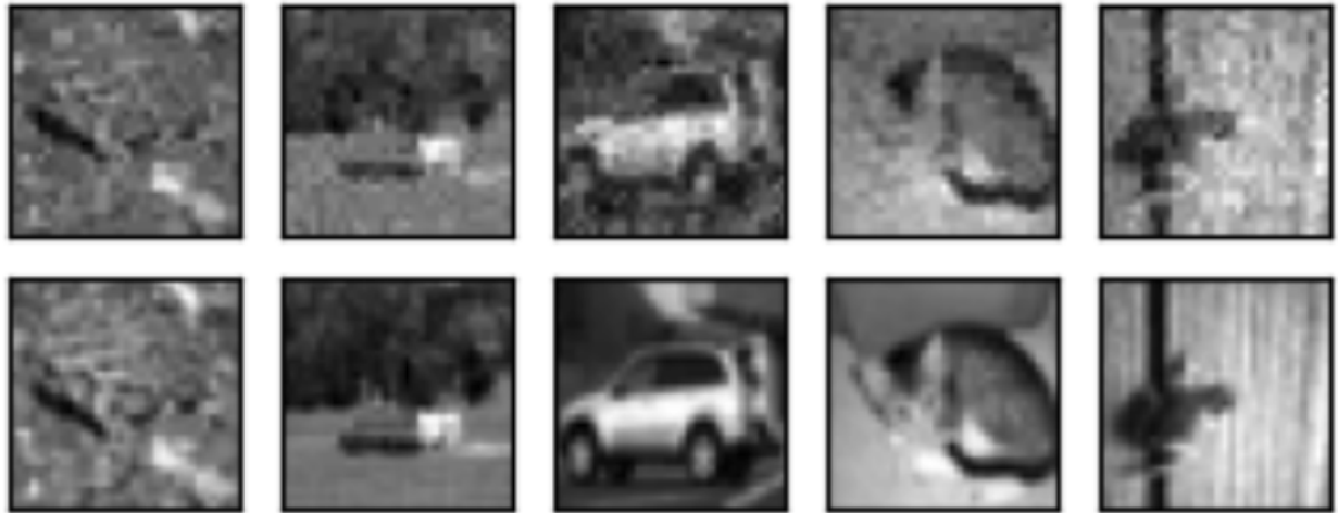
Figure 12: Example of reconstructed CIFAR10 images using the wavelet basis. Top row: reconstructed images. Bottom row: ground truth images. To reconstruct images we use 500 measurements and the number of layers optimized to get the best reconstruction possible.
