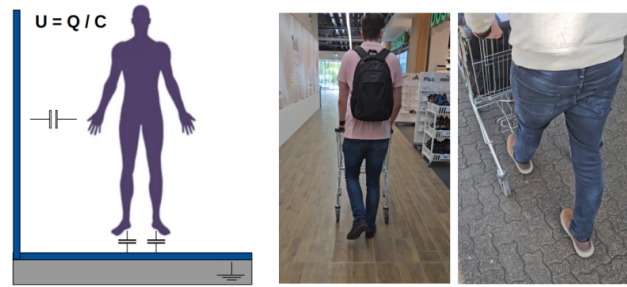
Figure 1: Left: Capacitor-like modeling of the human body describes the Body-area electric field, capacitive coupling through the air, shoe soles, and ground. U = human body surface potential, Q = human body surface charge, C = human body capacitance. Right: Data collection in/out of a shopping center while pushing a shopping trolley
