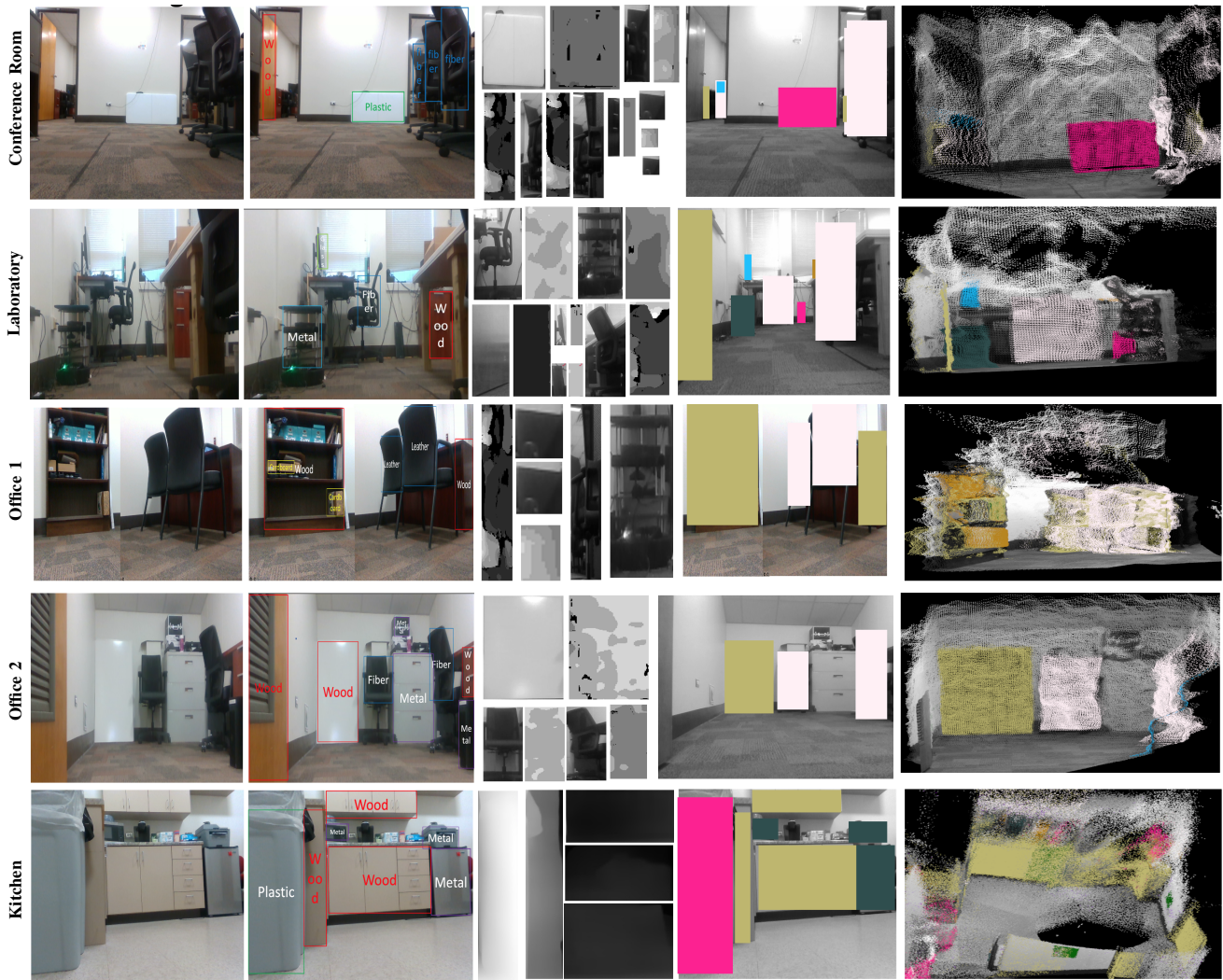
Fig. 6: Demonstration of sample outputs at various stages in our pipeline for the real-world robot RGB-D datasets. From left: RGB Image, ground truth material labels, segmented objects, material classification, and the final 3D clustering.
