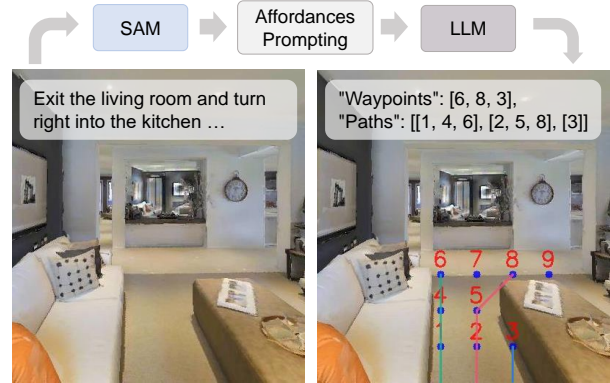
Figure 1: In discrete VLN, LLMs only need to perform high-level planning by selecting a view as the forward direction (left). For continuous environments, previous agents rely on collecting simulator data to train low-level policies. In this paper, we utilize multimodal foundation models and propose visual affordances prompting to predict low-level candidate waypoints and paths in a zero-shot setting (right).
