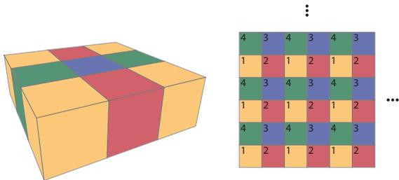
FIG. 6. Schematic of applying a series of  $\text{CZ}_{12}$  gates. Each colored cube represents an ancilla connected via  $\text{CZ}_{12}$  gate to the surrounding 12 qubits, as shown in Fig. 2c) in the main text. The Rydberg blockade means that the gates must be applied sequentially on differently colored cubes: (1) all yellow cubes, (2) all red cubes etc. Within a given color, the gates can be applied in parallel (i.e. all yellow cubes at the same time, etc).
