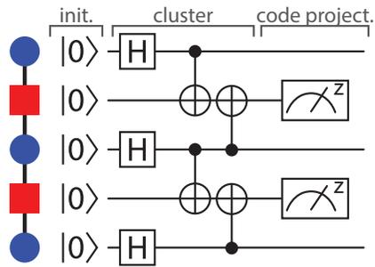
FIG. 7. The schematic of the quantum circuit using CNOT operators, equivalent to the circuit shown in Fig. 3(c). As before, this realizes an eigenstate of the X-cube model.
