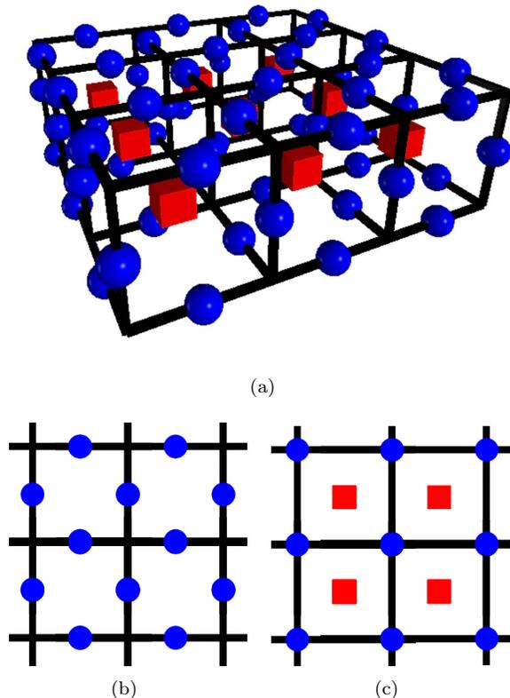
FIG. 1. (a) A Rydberg atom array composed of two species: the code qubits (blue) and ancilla qubits (red). This is achieved using alternating layers (b), (c) with the code qubits occupying the vertices (c) and the bond centers (b) of the square lattice, while the ancilla qubits inhabit the cube centers.
