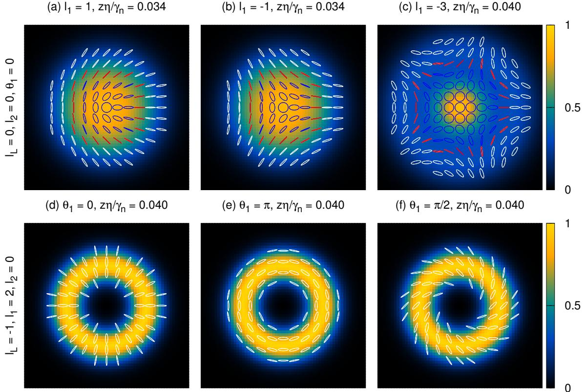
FIG. 3. This figure illustrates the intensity and polarisation distribution for various generated VB in a transverse plane. The blue, white, and red color ellipse corresponds to the left and right circular and linear polarisation. All other parameters are the same as Fig.2 except the beam waist for (a)-(c)  $w_L = 1.0w$  and  $w_1 = w_2 = 1.7w$  and (d)-(f)  $w_L = 0.8w$  and  $w_1 = w_2 = 1.0w$ .
