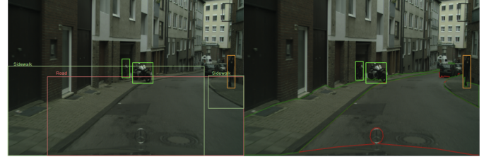
Fig. 6. Bounding box vs. semantic masks for road and sidewalk.
