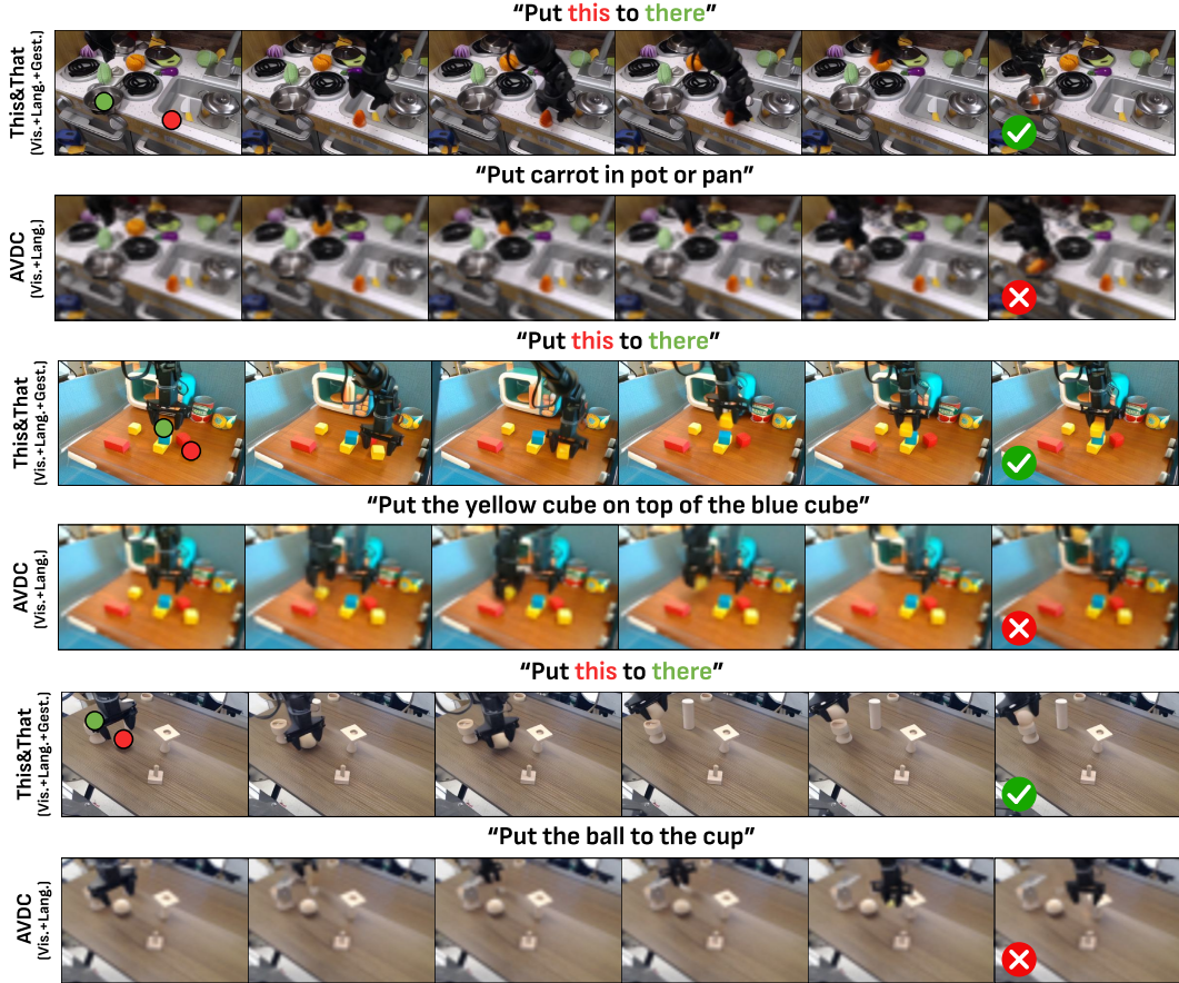
Figure 4: Video-based Planning Qualitative Results. We present three examples to compare This&That with AVDC [2]. The gesture locations are overlaid in the leftmost frame. Our method can generate action sequences effectively with higher visual quality, even when using deictic words.
