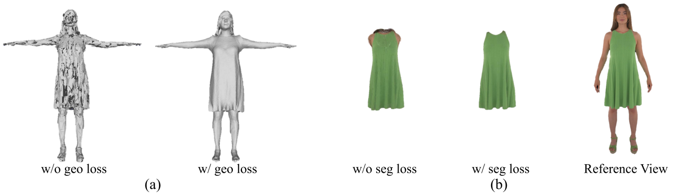
Fig. 6. (a) Ablation study on geometry regularization loss. Without geometry loss, the topology of the template meshes becomes chaotic and the surfaces become noisy. (b) Ablation study on segmentation loss. With segmentation loss, PICA can better distinguish between body and clothing, resulting in more stable animation and virtual try-on results.
