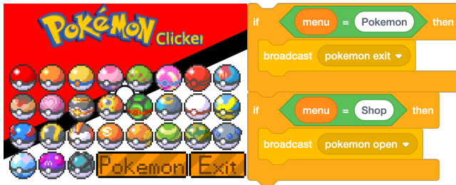
Figure 2: The PokéClicker game together with two conditions that are evaluated when pressing the Pokémon button and responsible for navigating the player to different menus.
