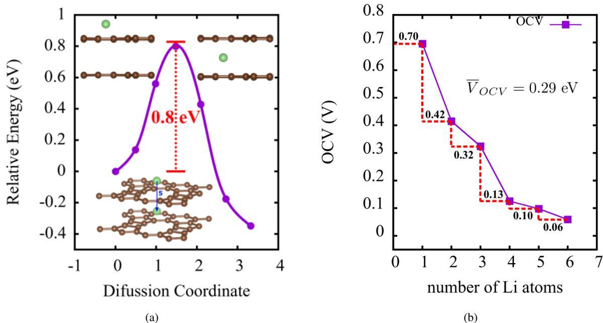
Figure 6: (a) Diffusion barrier of the Lithium atom into a TPDH-gr bilayer. These interlayer diffusions were considered only in the (D) region. (b) Open circuit voltage (OCV) as a function of the number ( $L$ ) of Li atoms adsorbed on TPDH-gr.
