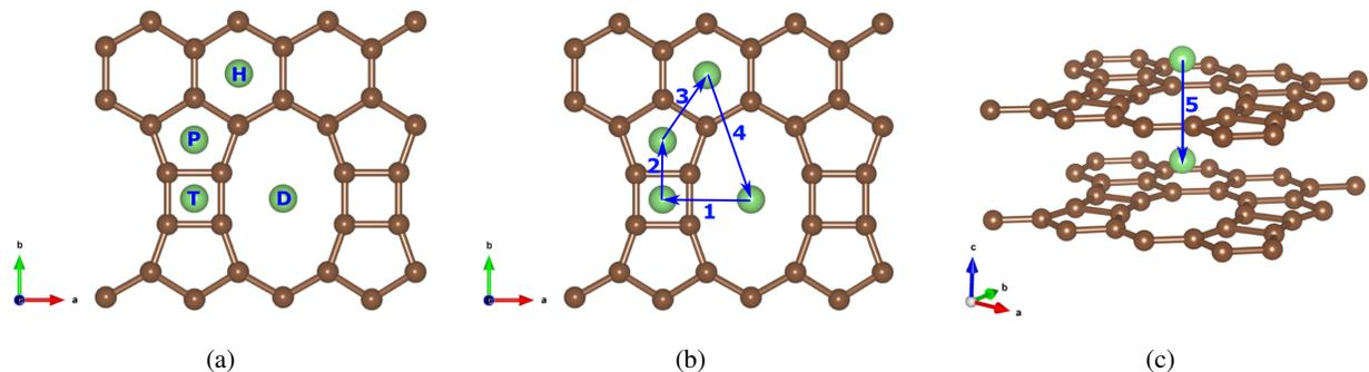
Figure 1: (a) Selected TPDH-gr regions for Li adsorption. (b) Investigated diffusion paths of Lithium ions on the TPDH-gr monolayer. (c) Investigated diffusion path in a TPDH-gr bilayer. These paths were chosen based on minimum energy pathways. See text for discussions.
