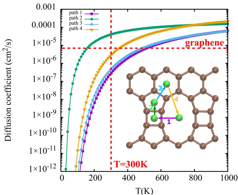
Figure 5: Diffusivity of Li atom over a TPDH-gr as a function of temperature ( $T$ ). Inset figure: The four diffusion paths of Li on the TPDH-gr are shown.
