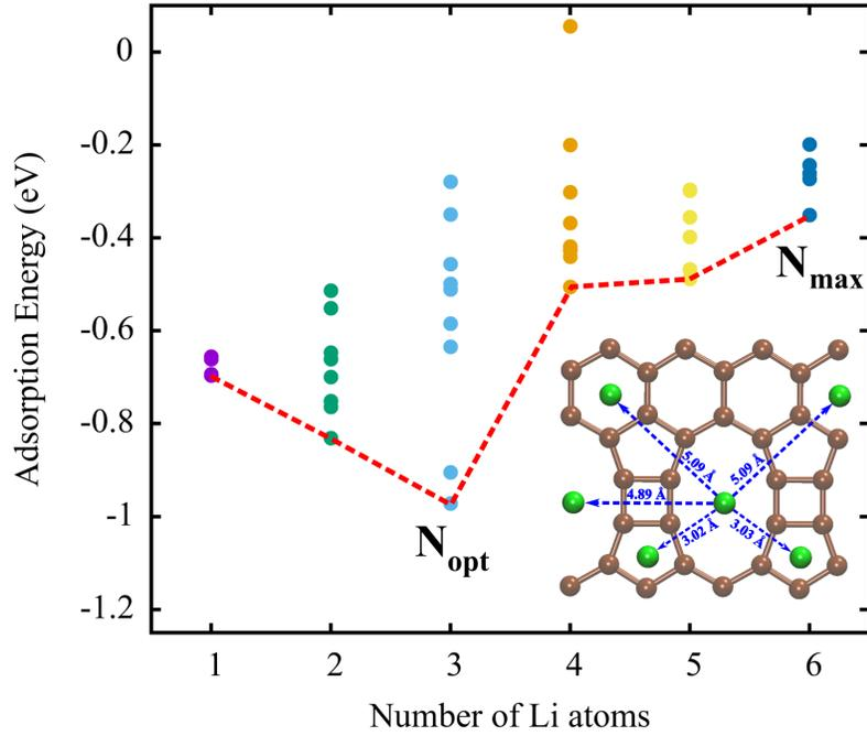
Figure 3: Adsorption energies  $E_{ads}^{bcc}$  (eV) as a function of the number  $N$  ( $N=1,2,\dots,6$ ) of Li atoms. Inset figure: Configuration of TPDH-gr with  $N=6$  Li atoms, showing that the distance between Li atoms is  $> 2.80 \text{ \AA}$  to prevent clustering.
