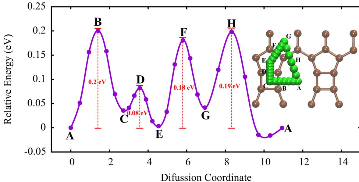
Figure 4: Diffusion energy barriers of the Lithium atom on the surface of TPDH-gr. Inset figure: all intermediate Li images for each diffusion path are shown.
