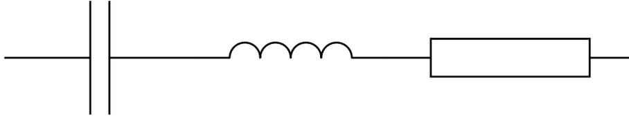
Figure 2.1: LCR circuit
