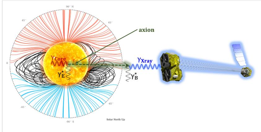
**Fig. 1:** NuSTAR spacecraft [18] (right) searching for X-ray photons (blue line) from axion-to-photon conversion in the solar atmosphere (left). Axions (green dashed line) are created in the hot plasma of the solar core via the Primakoff effect due to the presence of electric fields ( $\gamma_E^*$ ) and get back-converted into X-ray photons by means of the inverse-Primakoff effect in the presence of the magnetic fields ( $\gamma_B^*$ ) in the solar atmosphere [19].
