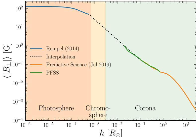
**Fig. 11:** Our fiducial magnetic field model (blue, dashed black, and orange) derived from the PSI simulation for the 2019 eclipse in comparison to the PFSS model for the day of NuSTAR observations (green). The two models are in excellent agreement in the range of altitudes where the PFSS result is reliable.
