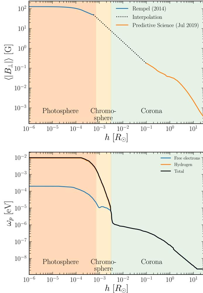
**Fig. 3: Top:** Modeling of the transverse component of the solar atmospheric magnetic field: Rempel [55] (blue line), Predictive science [56] (orange line), and power-law interpolation between both models (dashed black line). **Bottom:** Contributions to axion plasma frequency from free electrons (blue line), hydrogen (orange line), and total added contribution (black line). **In both view-graphs:** shaded regions for the photosphere (orange), chromosphere (yellow), and corona (green).
