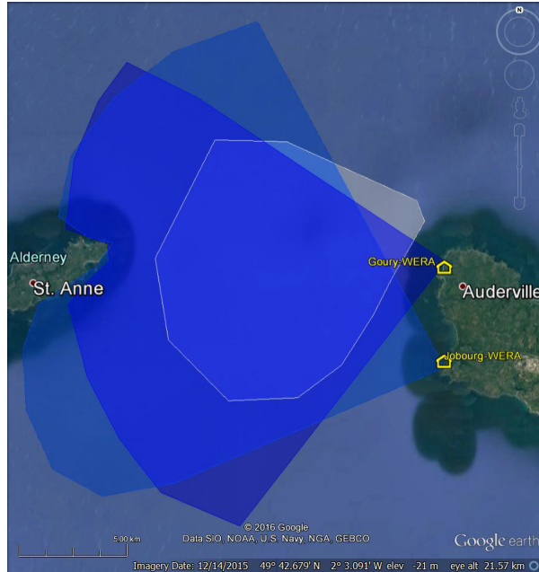
Fig. 1 Locations of the two HF radar sites: Gourey-WERA and Jobourg-WERA and their spatial coverage (blue patterns) with the common region (white/gray contours) (Helzel et al, 2017).
