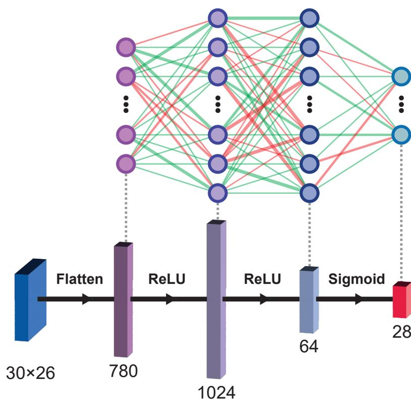
Supplementary FIG. S2. **Architecture of the spectral prediction network.** The 3-layer multi-label classification neural network model for mode visualisation. For the input and hidden layers (except the last hidden layer), a ReLU activation function is used. A sigmoid activation function is applied at the last hidden layer to produce a one-hot encoded mode spectral profile. The number of nodes in each layer is shown at the bottom
