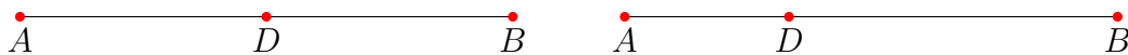
FIGURE 4. The new node on an edge AB . (left): A \neq Q_i and B \neq Q_i (midpoint); (right): A = Q_i ( |AD| = \kappa_{Q_i}|AB| , \kappa_{Q_i} < 0.5 ).
