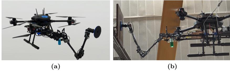
**Fig. 1:** Proposed coaxial tilting octa-rotor equipped with a robotic arm. Snapshot in laboratory (a) and during task execution (b).
