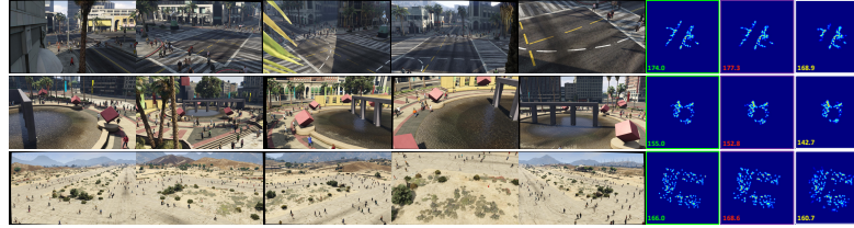
Fig. 3: Qualitative Results. The figure visualizes 3 challenging scenarios on the CVCS benchmark. Regarding each sample, the visualization includes the multi-view images (with 5 views), ground truth density, density obtained with the MV volume aggregation module , and density estimated without this module .
