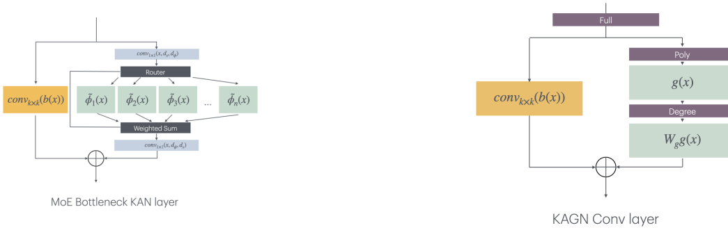
Figure 2: Bottleneck Kolmogorov-Arnold Convolutional Mixture of Experts. The router and experts are placed between bottleneck convolutions, and each expert is a \tilde{\varphi} set of univariate functions. We use sparsely-gated mixture-of-experts [15].
