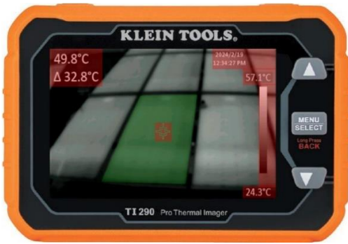
Fig. 2. An infrared thermography camera used for data collection [36]. The image shows masked overlay information regions in red and the most prominent PV panel in green.
