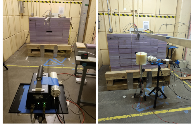
Fig. 1. Experimental configuration. P385 neutron source is surrounded by a carbon steel and borated polyethylene collimator [7]. A neutron exit aperture that has a tapered shape in the horizontal plane is created in the steel cylinder and polyethylene block with an opening angle of 17.5 degrees and a height of 2". The left figure shows the BTI N-Probe and an EJ-410 detector at 3 m distance. The right figure shows the NNS and an EJ-410 detector placed at 1 m distance from the source. In both configurations, another EJ-410 detector is on the floor under the P385 and the collimator, covered by a layer of 2"-thick lead bricks, which is not shown in the picture. Between the P385 and the EJ-410 on the floor, there is a cylindrical cavity in the collimator and moderator, directed towards this detector.
