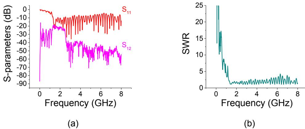
Figure 6. Experiments: (a) S-parameters in dB and (b) Standing wave ratio (SWR) of  $S_{11}$ .
