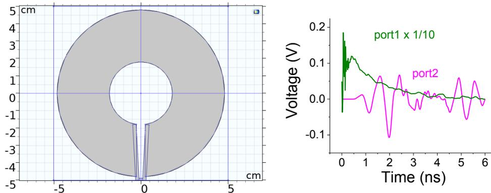
Figure 9. Simulations: Slanted feeding transmission line to solid loop and its voltage response.
