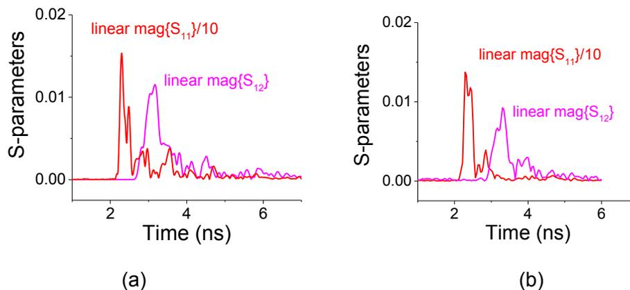
Figure 7. Experiments: linear magnitude of the S-parameters as a function of time (one way). The full width of the signal at half maximum amplitude (FWHM) of the  $S_{11}$  was 260 ps (accounting for the entire pulse) whereas the FWHM of the  $S_{12}$  was 380 ps. A 1 ns propagation delay between the recorded pulses is also noted. (b) Solid thick loop (Fig. 4): FWHM of the  $S_{12}$  was 380 ps, as well.
