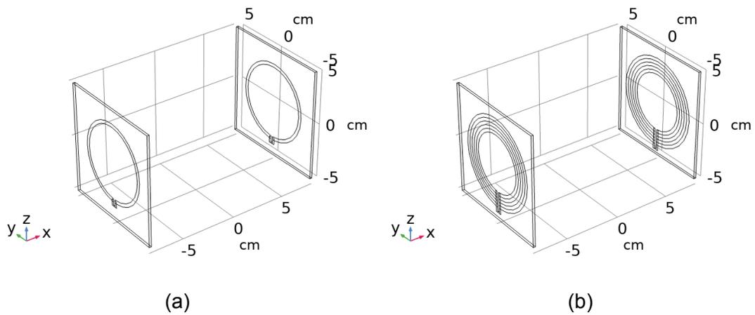
Figure 2. Simulations: a pair of single (a) and 3-loop antennas (b) – the transmitter is on the right and the receiver is on the left.
