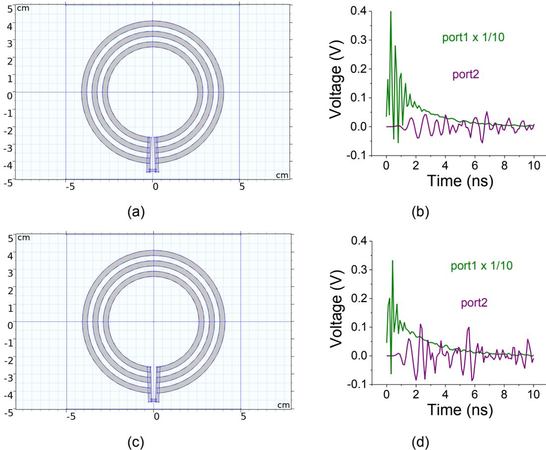
Figure 8. Simulations: (a,c) Slanted feeding transmission lines and their voltage response (b,d). Note the reflection effect at 6 ns.
