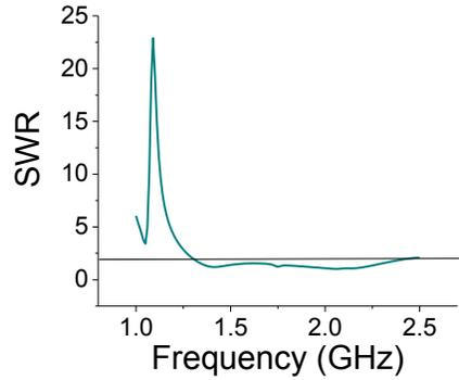
Figure 3. Simulations: standing wave ratio (SWR) for 3-loop, equally spaced antenna. The horizontal line is placed at SWR=2 and alludes to a bandwidth of more than 1 GHz.
