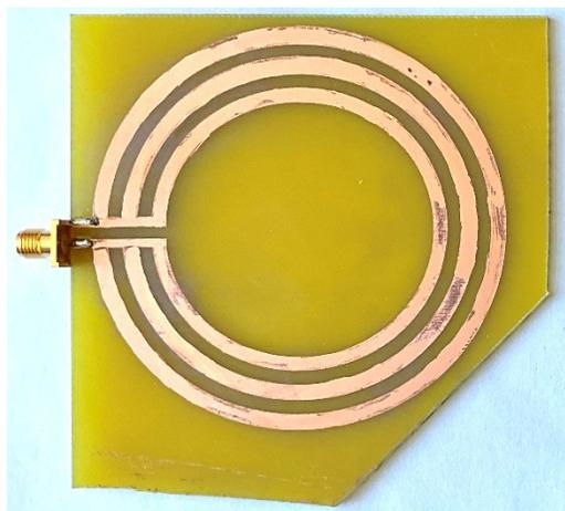
Figure 5. Experiments: the antenna on FR4 dielectric and its SMA connector. The cut in the FR4 is the result of fabricating two antennas on the same substrate.
