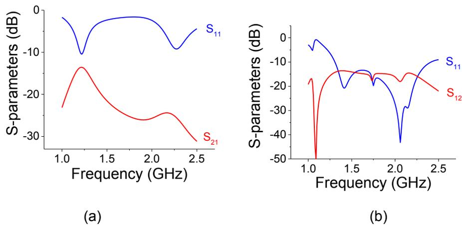
Figure 2. Simulations: (a) S-parameters for a single loop antenna. (b) S-parameters for 3-loops, equally spaced antenna
