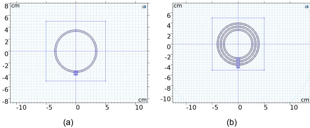
Figure 1. Simulations: (a) A single loop antenna. (b) 3-loop antenna. The central loop has the same dimensions as the loop in (a).
