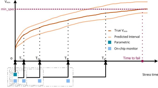
Figure 1:  $V_{min}$  prediction flow
