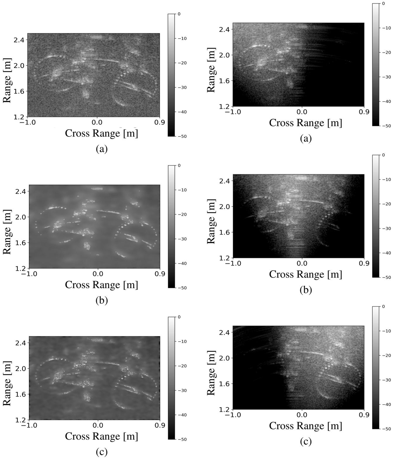
Fig. 14. a) the noisy image, b) the de-noised image, c) the de-noised image by applying the de-noising technique given in (5) to the result of the complex dual apodization method shown in Fig. 13-(c).
