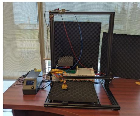
Fig. 7. The radar system as well as the motorized scanner to create the synthetic aperture.
