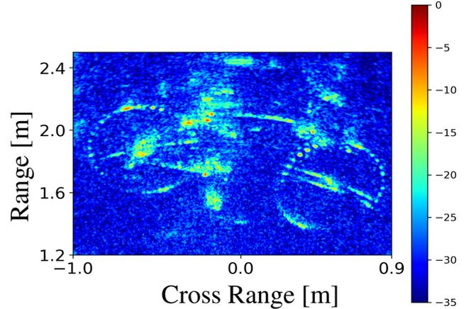
Fig. 10. The reconstructed image after applying Hamming window in both the range and cross-range directions.
