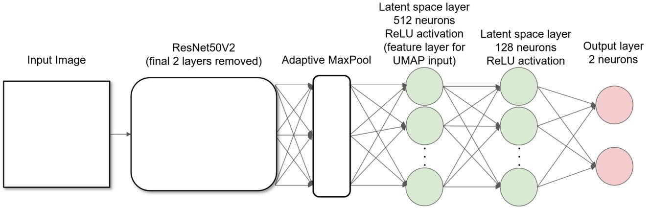
**Figure 2.** The input  $256 \times 256$  image serves as the initial input to the pre-trained ResNet50V2 model. The last two layers of the pre-trained network have been replaced with an adaptive max pooling layer. This is then followed by two fully connected layers, consisting of 512 and 128 neurons, respectively. Activation of these layers is achieved through the ReLU activation function. In this work, the output layer utilized is actually the 512 neuron layer.
