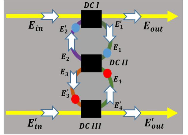
FIG. 8. Schematic of the  $\mathcal{PT}$ -Symmetric Ikeda Map. The **yellow-colored** blocks are the passive input and output channels and the **black-colored** blocks, labelled as *DC I*, *DC II* and *DC III*, are the 50:50 directional couplers. The amplifiers are colored **red** and the attenuators are colored **blue**. The feedback loops with saturation nonlinearity are colored green, purple and brownish.
