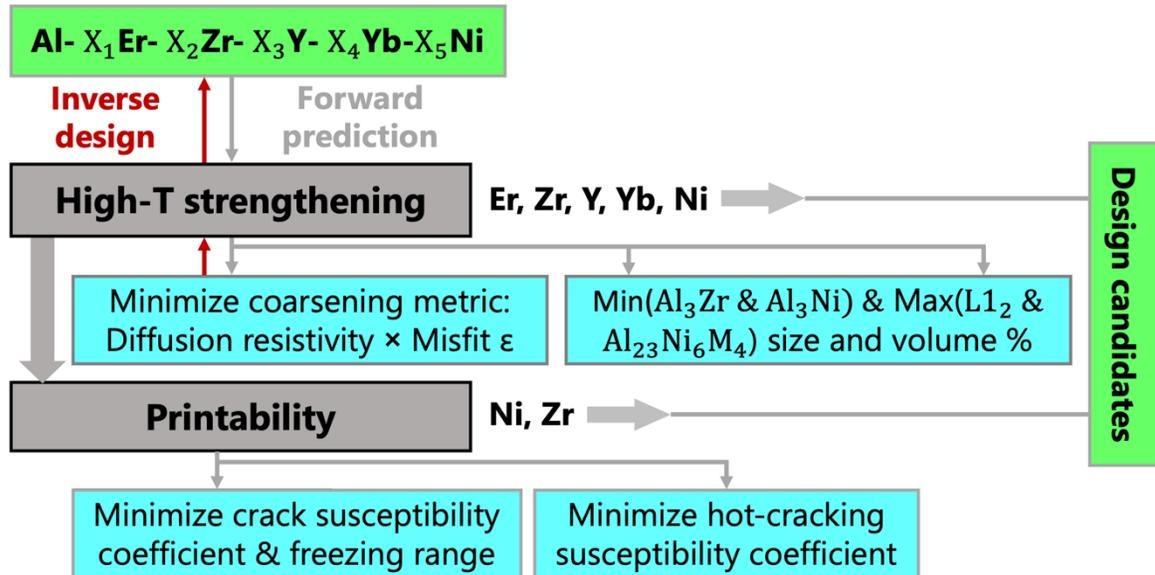
Fig. S1. Flow diagram and design approaches for measuring structure parameters. The composition is inversely designed for the primary goal of minimizing the coarsening metric of  $L_{12}$  phases. All other microstructural features are forward predicted and work as constraints for the inversely designed composition.
