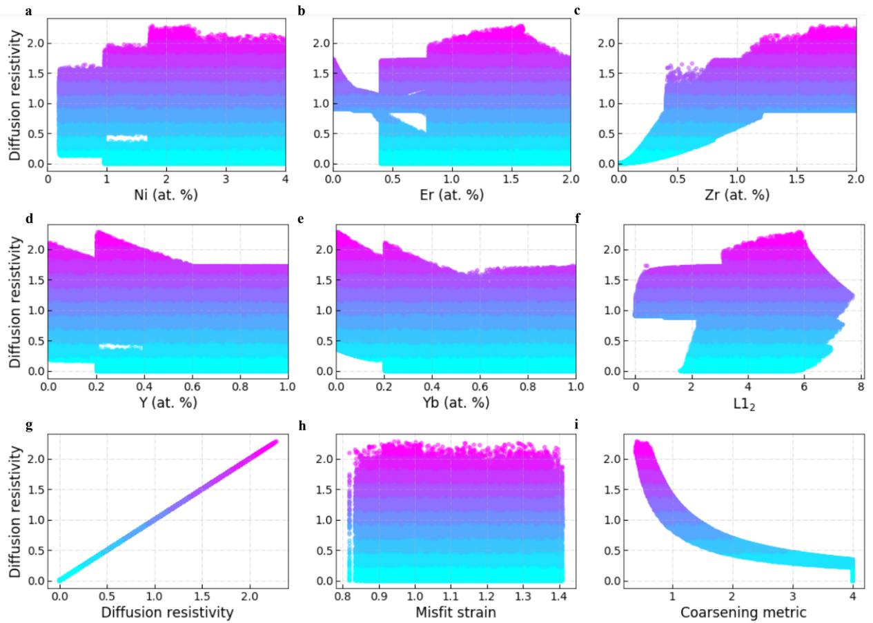
Fig. S5. Distribution of diffusion resistivity with respect to studied parameters. Increasing Zr has the greatest influence on increasing diffusion resistivity.
