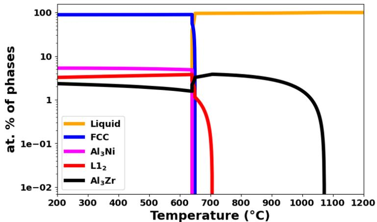
Fig. S3. CALPHAD simulation of phase at. % with respect to temperature for our designed Al-Ni-Er-Zr alloy.
