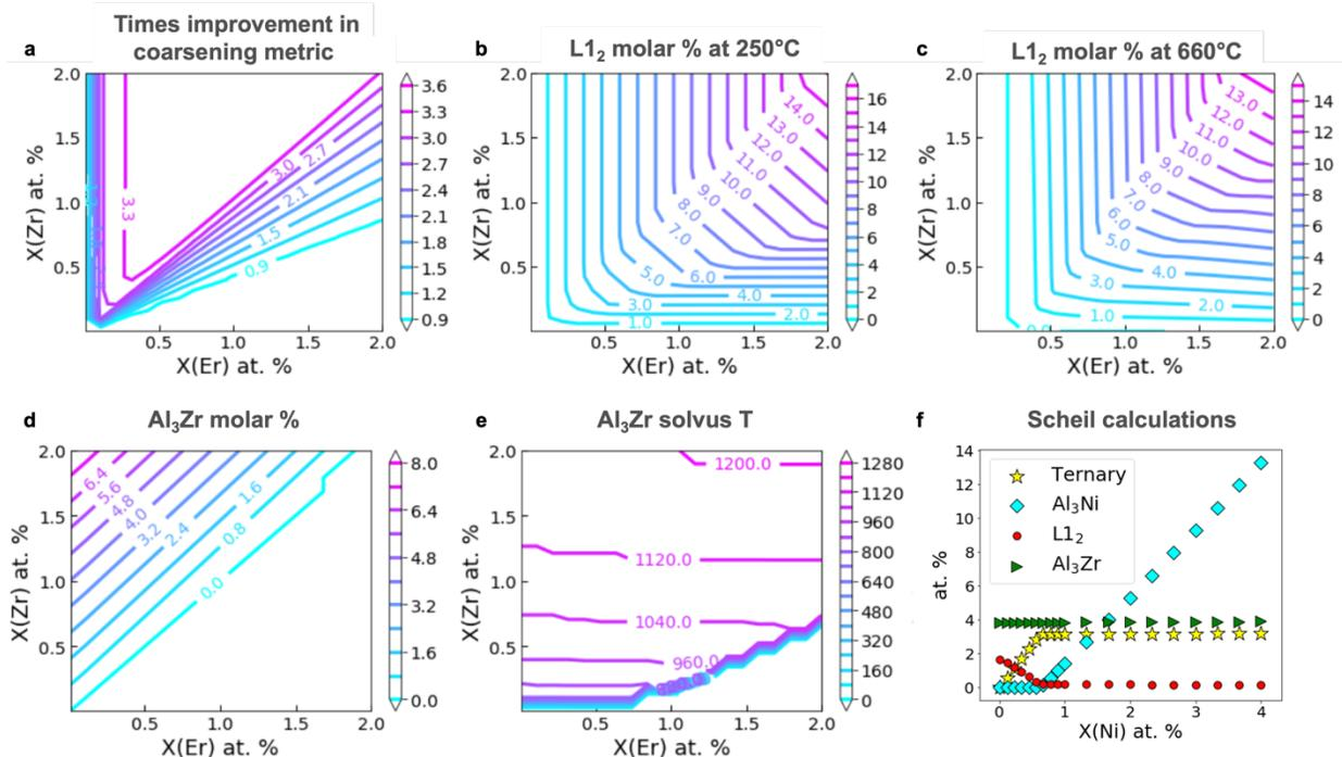
Fig. 4. a-f) Forward prediction of structural parameters with respect to Er and Zr at. %. Each structural feature defines a limit on the Er/Zr content. f) At. % of different phases produced by changing the Ni at. % in Scheil simulations (Er = 0.4 at. % and Zr = 1 at. %). The reduced space of “a-f” only with respect to Er and Zr and “g” only with respect to Ni, are explained in the Results and Discussions Section.
