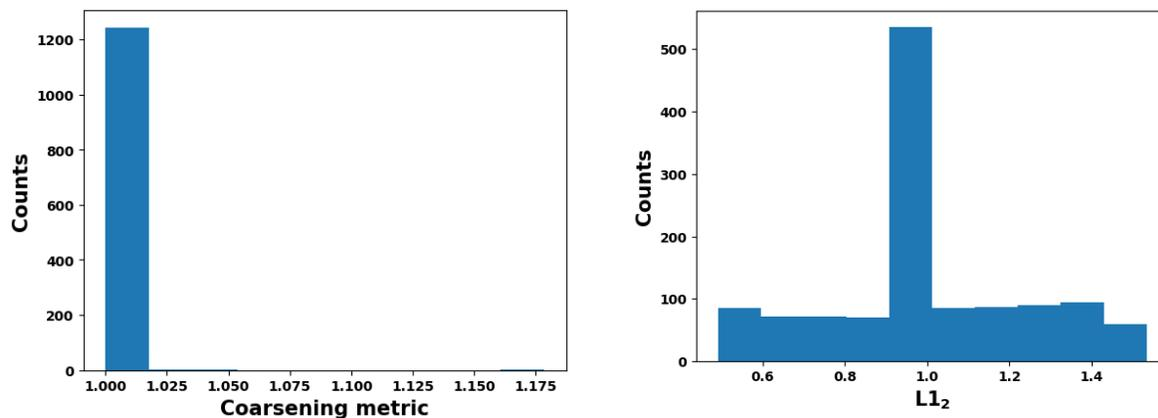
Fig. S10. Histogram of the coarsening metric and  $L1_2$  at. % of 1250 designs varied from the ML-optimized design by up to 50% change in composition, normalized against the ML-optimized design. Both descriptors are highly stable under these variations.
