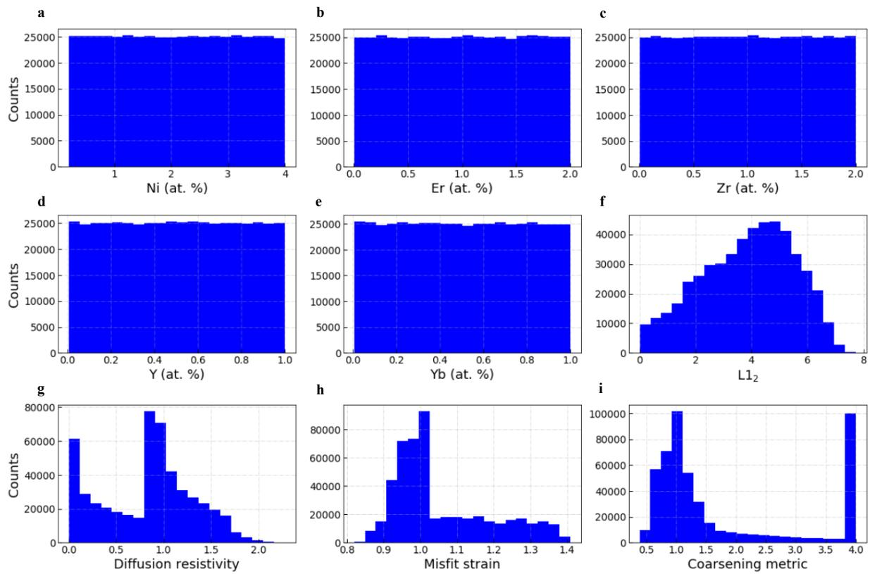
Fig. S4. Distribution of at. % for alloying elements and normalized target properties (i.e.,  $L_{12}$ , diffusion resistivity, misfit strain ( $\epsilon$ ), and coarsening metric) for 500,000 random compositions. Target properties are normalized with associated values from the benchmark printable Al alloy. Coarsening metrics  $> 4$  are assigned 4.
