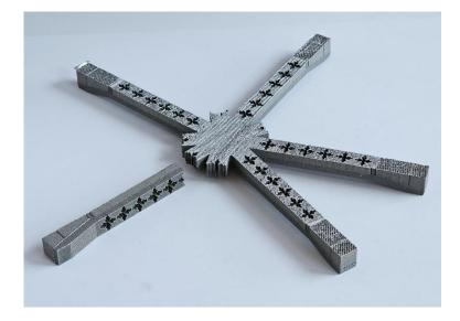
Fig. 2. A spider-inspired ultrasonic device manufactured by using the DMLS method.
