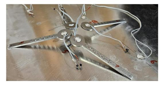
Fig. 13. Four ultrasonic devices bonded to an aluminium plate.
