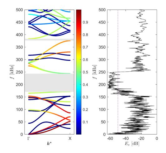
Fig. 7. The band gap in the laser-cut aluminium spider's leg: numerical and experimental analysis.
