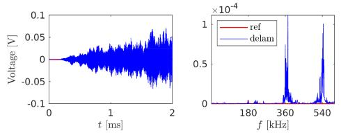
Fig. 12. Time and frequency domain signal response at the sensor on the ultrasonic device made of steel.
