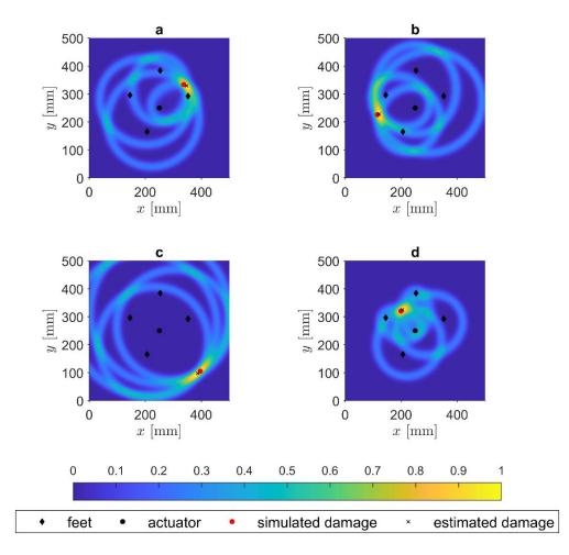
Fig. 18. Damage maps obtained by the time of arrival method (ellipse method) for simulated damage at a) position 6, b) position 7, c) position 8, d) position 9.
