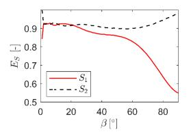
Fig. 5. Signal energy  $E_S$  dependence on the angle  $\beta$  for signals transmitted to point S<sub>1</sub> on the leg and S<sub>2</sub> on the surface of the plate, respectively.
