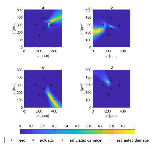
Fig. 17. Damage maps obtained by the method of difference in wave arrival (hyperbole method) for simulated damage at a) position 6, b) position 7, c) position 8, d) position 9.
