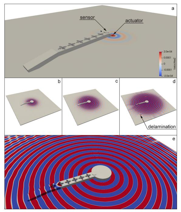
Fig. 10. Ultrasonic guided wave propagation in a plate with a delamination and ultrasonic device with embedded PCs at the time frames: a)  $31.2 \ \mu$ s, b)  $46.9 \ \mu$ s, c)  $140.6 \ \mu$ s, d)  $187.5 \ \mu$ s, e)  $250 \ \mu$ s.
