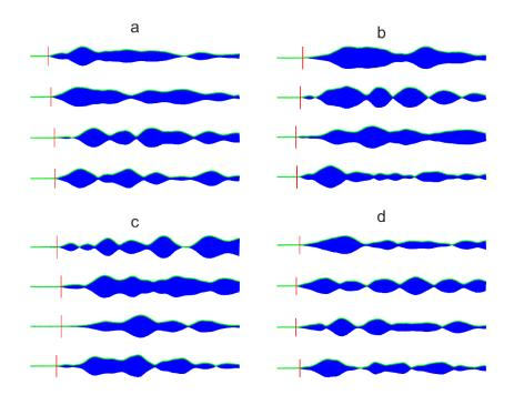
Fig. 16. Estimated time of arrivals (red lines) in signals with applied Hilbert envelope (green) registered at four legs (blue): a) simulated damage at position 6, b) simulated damage at position 7, c) simulated damage at position 8, d) simulated damage at position 9.
