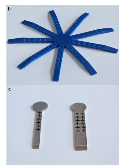
Fig. 3. Prototypes of ultrasonic devices: a) spider-inspired device laser-cut from aluminium alloy sheet, b) 3D-printed polymer spider-like geometry, c) laser-cut steel legs.
