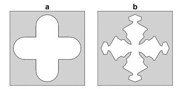
Fig. 6. Unit cell geometries with grey representing solid material and white representing the cavity: a) cross-like shape used in laser cut aluminium spider (see Fig. 3a), b) optimised cavity shape used in 3D-printed polymer spider (see Fig. 3b) and laser cut steel legs (see Fig. 3c).
