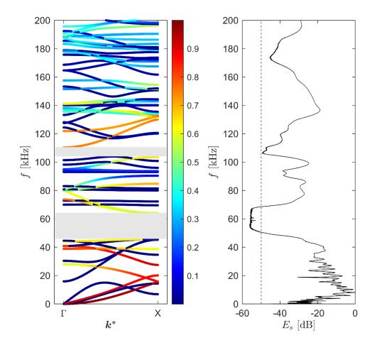
Fig. 8. The band gap in the 3D-printed polymer spider leg: numerical and experimental analysis.
