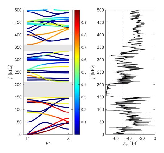
Fig. 9. The band gap in the laser-cut steel spider's leg: numerical and experimental analysis.
