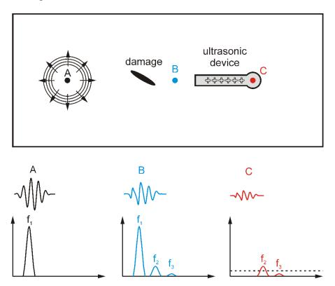
Fig. 1. Metamaterial-aided defect detection by utilization of higher harmonics.
