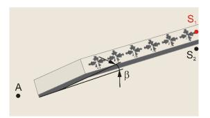
Fig. 4. Parametric studies of guided wave actuation at point A and sensing at points S<sub>1</sub> and S<sub>2</sub>.
