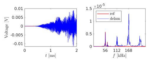
Fig. 11. Time and frequency domain signal response at the sensor on the ultrasonic device made of polymer.
