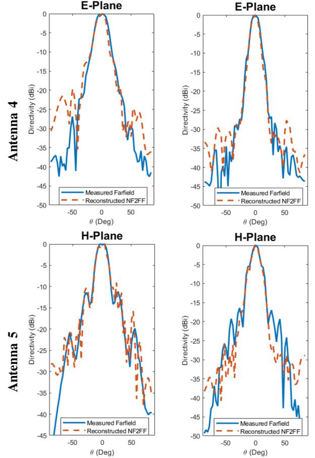
Fig. 5. Comparison of the measured (fully-sampled) and reconstructed (3x downsampled) far-field patterns in both E and H plane. Antenna 4 and 5 are two horn antennas with an operating frequency at 75 GHz and 90 GHz.
