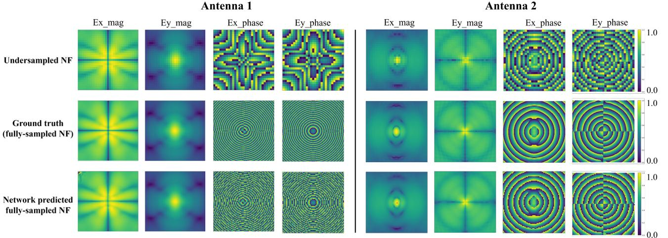
Fig. 3. Comparison of the network’s capability to conduct near-field super-resolution on data with a downsampling factor of 3. Undersampled NF and ground truth represent the low-resolution input and the fully-sampled, high resolution output of the network, with predicted NF showing the network’s estimations based on low-resolution data. Antenna 1 is a horn antenna working at 8.4 GHz, while the antenna 2 operates at 3 GHz as a Yagi antenna. The range of values is [0, 1] as shown on the color bar.
