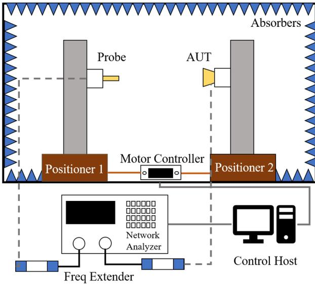
Fig. 7. The NF measurement setup used in this experiment. The system consists of a motor-controlled motion stage hosted on a vibration-absorbing optical table surrounded by absorbers. The characterization probe and the AUT are connected by a 2-port VNA and frequency extenders to acquire near-field data.
