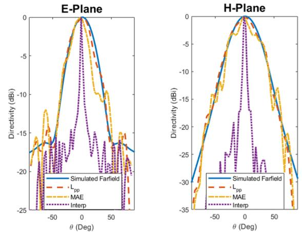
Fig. 8. Comparison of the reconstructed far-field pattern of antenna 1 based on different super-resolution strategies and loss functions used to train the NFS-NET. The simulated far-field pattern (ground truth) is added for comparison.
