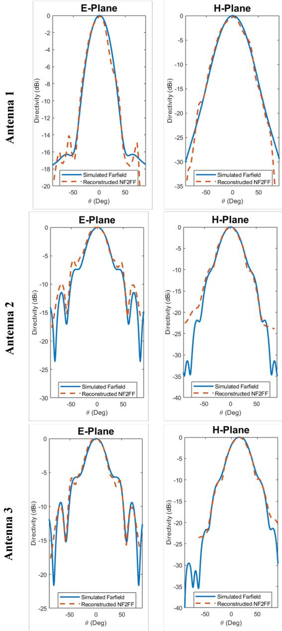
Fig. 4. Comparison of the simulated (fully-sampled) and reconstructed (3x downsampled) far-field patterns in both E and H plane. Antenna 1 and 2 represent the same antennas in the near-field super-resolution examples, with antenna 3 demonstrating a modified version of antenna 2 tilted at an angle of  $15^\circ$ .
