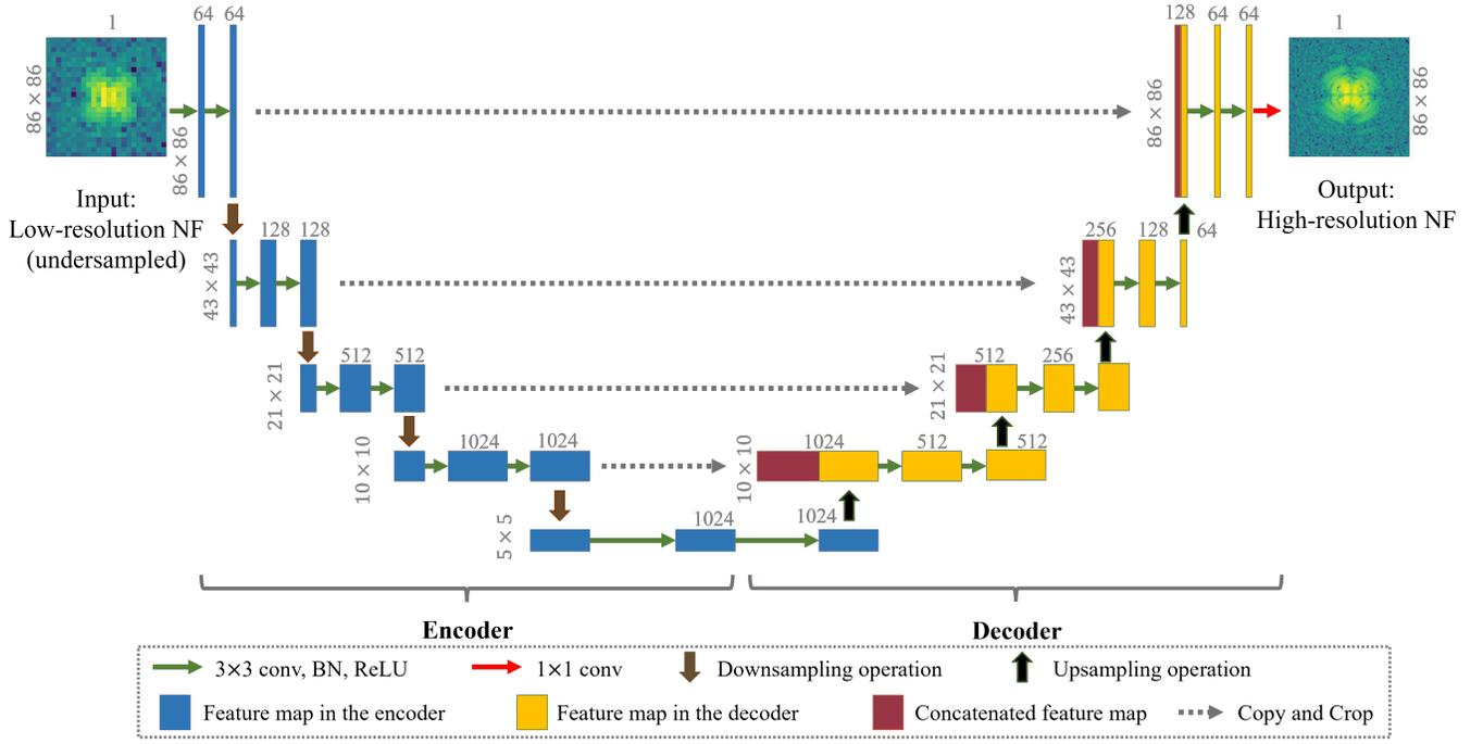
Fig. 2. The overall architecture of NFS-Net. It consists of an encoder, a decoder, and skip connections between them to preserve high-resolution features and extract informative content. Detailed dimensions and channel sizes can also be found in numerical annotations.
