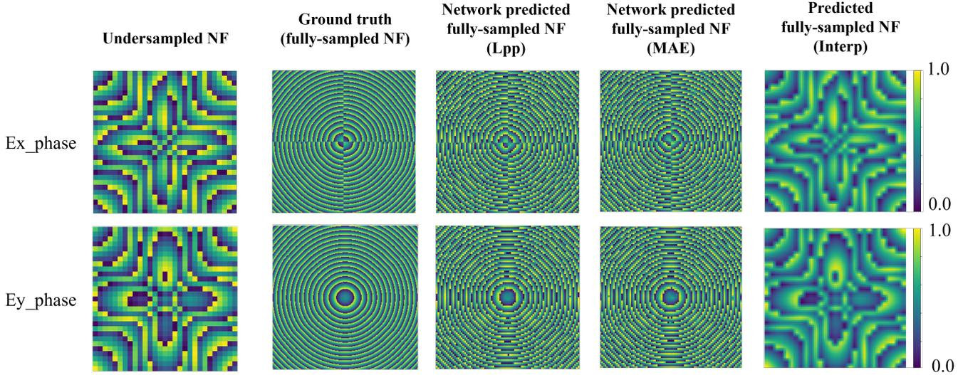
Fig. 6. Comparison of the restored near-field phase maps of antenna 1 based on different super-resolution strategies and loss functions used to train the NFS-Net, with reference to the fully-sampled NF map as ground truth.
