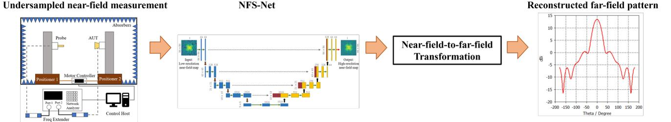
Fig. 1. The workflow of the proposed end-to-end fast NF antenna measurement. It starts with the undersampled measurement of  $E_x$  and  $E_y$  in the near-field of the AUT. The undersampled near-field data map is then fed into the NFS-Net to restore its fully-sampled counterpart, which is then further processed by the NF2FF algorithm to reconstruct the far-field radiation pattern.
