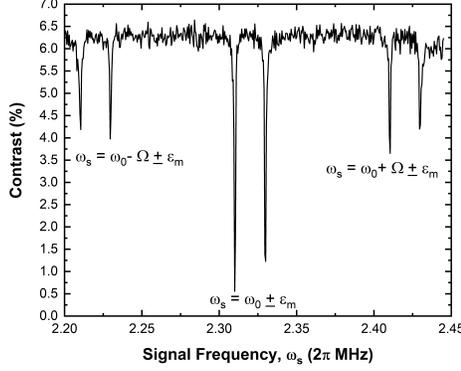
**Fig. 3 Sensor resonances** Sensor response as a function of signal frequency  $\omega_s$ , displaying six sensor resonances centered on the electron spin transition,  $\omega_0 = 2.32$  GHz. The contrast was sampled after exposing the  $V_B^-$  ensemble to a CCDD pulsewidth of  $T_M W = 950$  ns. The applied signal had an amplitude of  $g_x = 0.8$  MHz and phase  $\phi_s = 0$ . Drive phase was omitted,  $\theta_m = 0$ .
