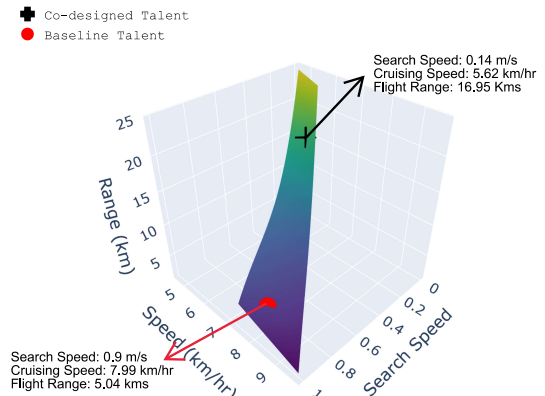
Fig. 5: Talent Pareto front represented by Polynomial Regression applied to computed Pareto solutions obtained by multi-objective optimization of Talents; limits of talents captured with quantile regression.
