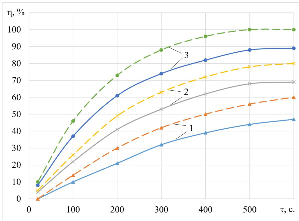
Figure 4. Crystallization kinetics of paraffin drops with a diameter of  $100\mu\text{m}$  depending on the overheating temperature and the exposition time in the superheated state at  $2^\circ\text{C}$  and supercooling: 1 –  $15^\circ\text{C}$  superheating; 2 –  $10^\circ\text{C}$  and 3 –  $5^\circ\text{C}$ .
