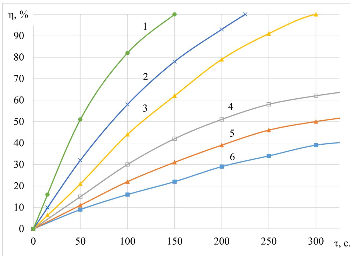
Figure 3. Kinetics of paraffin (1, 2 and 3) and salol (4, 5 and 6) drops crystallization with diameters of 100 $\mu\text{m}$  (3, 6), 150 $\mu\text{m}$  (2, 5) and 200 $\mu\text{m}$  (1, 4) with supercooling temperature of 3 $^{\circ}\text{C}$  and 10 $^{\circ}\text{C}$ , respectively.
