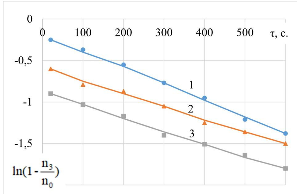
Figure 5. The change of the parameter  $\ln(1 - \frac{n_3}{n_0})$  on  $\tau$  (Eq. (7)) for paraffin drops with a diameter of  $100\mu\text{m}$  supercooled by  $2^\circ\text{C}$ , overheated by: 1 –  $15^\circ\text{C}$ , 2 –  $10^\circ\text{C}$  and 3 –  $5^\circ\text{C}$
