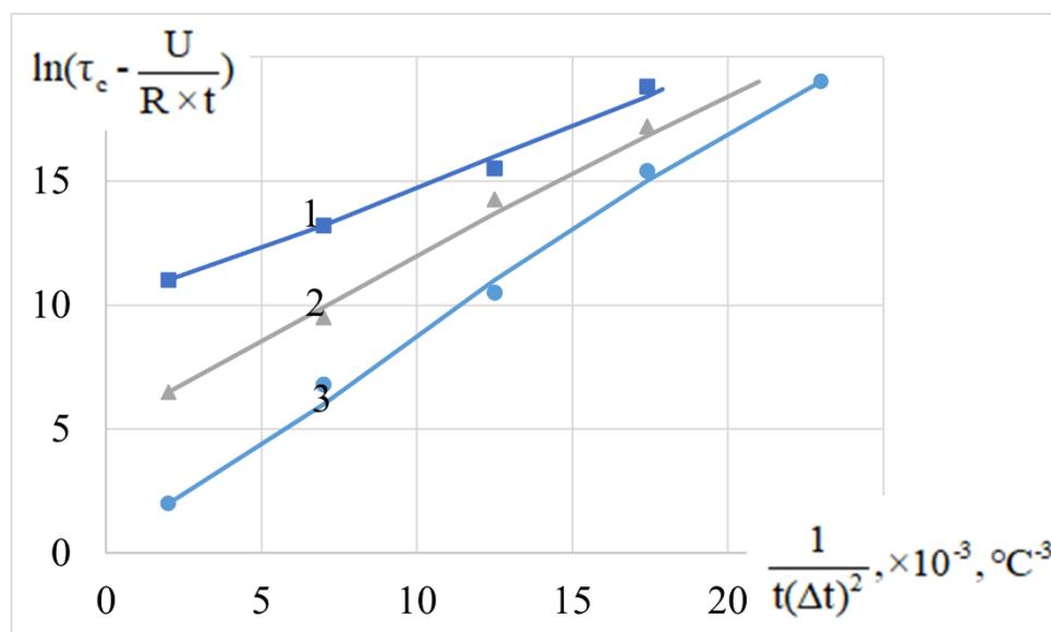
Figure 6. The change of the parameter  $(\ln \tau_c - \frac{U}{Rt})$  on  $\frac{1}{t(\Delta t)^2}$  (Eq. (12)) for paraffin drops with a diameter of 100  $\mu\text{m}$ , superheated by 5 $^{\circ}\text{C}$ , with supercooling of 2 $^{\circ}\text{C}$
