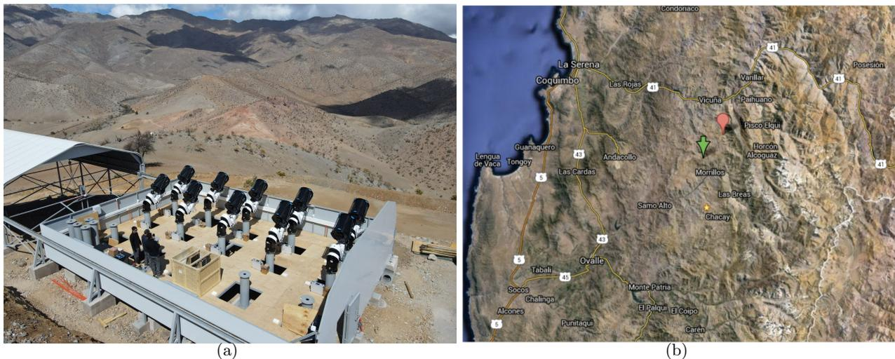
Figure 3. (a) A bird’s eye view of 7DT at El Sauce Observatory in Chile. The picture shows 10 units of DR500 installed as of September 2023. (b) The location of the El Sauce Observatory is indicated with a yellow star. Green and Orange arrows show the respective locations of CTIO and Cerro Pachon.
