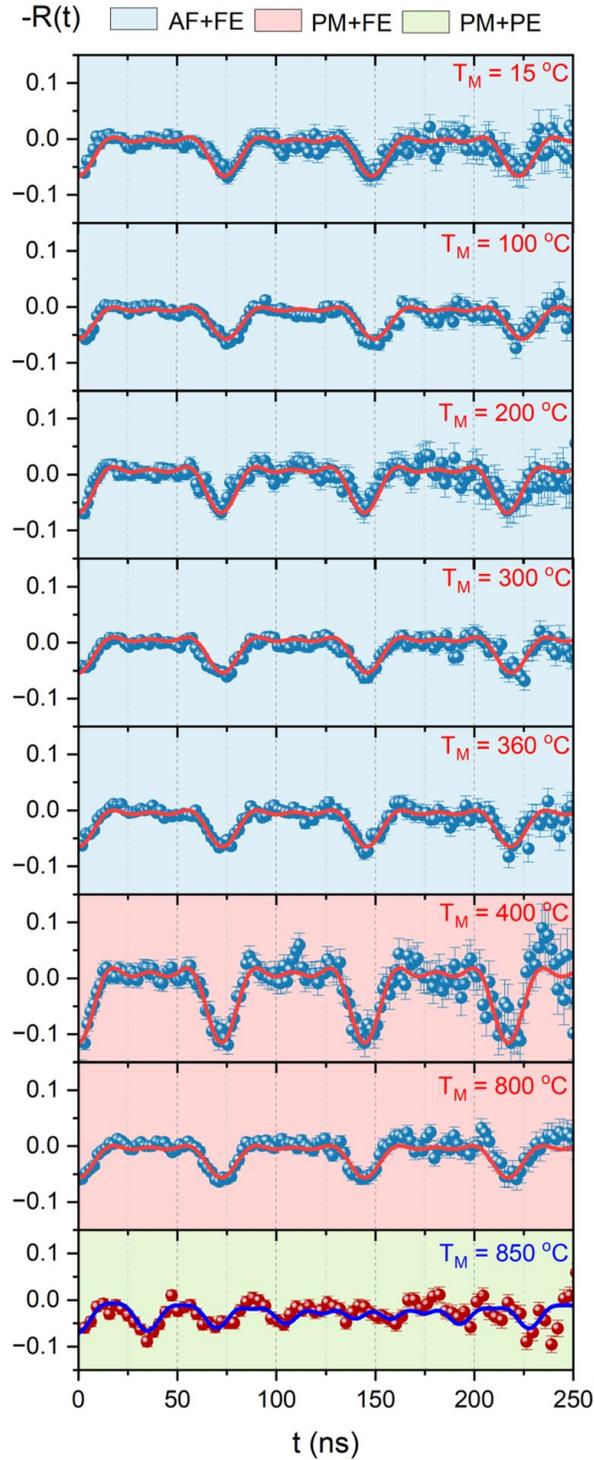
**Figure 4.** The temperature-dependent TDPAC spectra  $R(t)$  were fitted using the PACfit software<sup>12</sup>. The spectra at 15 °C, 200 °C, 400 °C, and 850 °C were obtained using the KATAME<sup>40</sup> spectrometer whereas other spectra were measured at K1<sup>41</sup>. Blue, red, and green backgrounds denote spectra in the antiferromagnetic and ferroelectric (AF + FE), paramagnetic and ferroelectric (PM + FE), and paramagnetic and paraelectric (PM + PE) temperature ranges, respectively.
