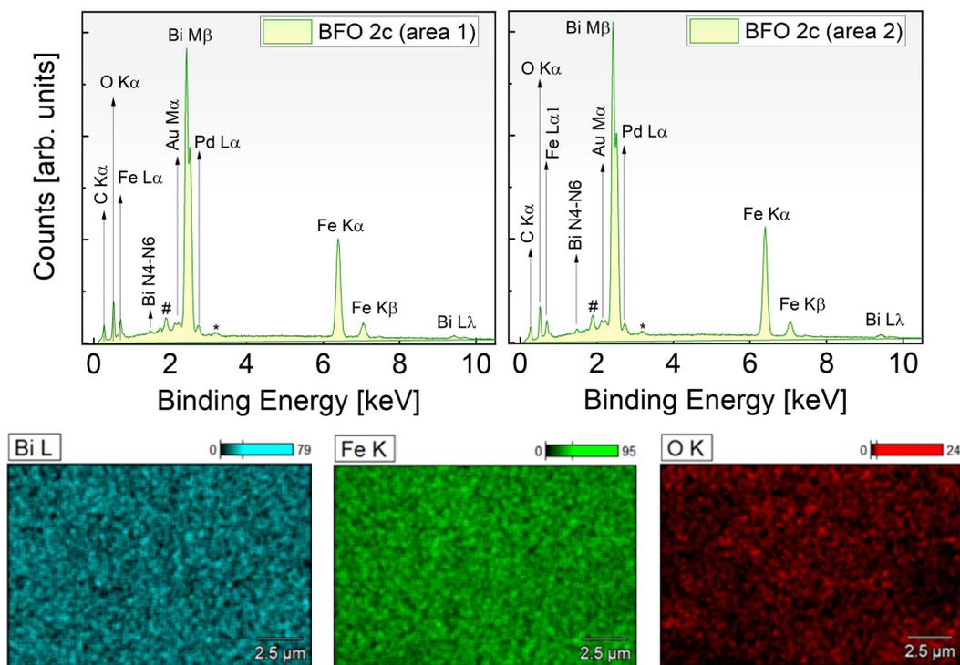
**Figure S4.** The EDXS spectra and elemental mapping of sample BFO2c (fresh sample) are shown. The unassigned peaks (#, \*) might have originated from the sample holder and carbon residues of the carbon tape that was used to attach the sample to the sample holder.
