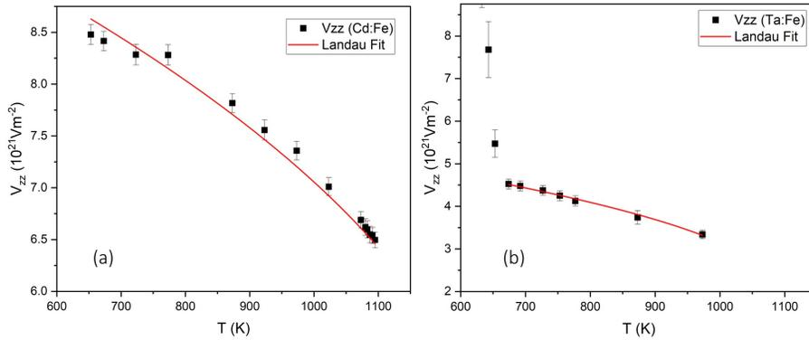
**Figure S9.** (a) Temperature dependence of  $V_{zz}$  at the Fe site using <sup>111</sup>In<sup>11</sup> and (b) <sup>181</sup>Hf probes<sup>23</sup>. The data was re-fitted using the formula (s9), which follows the Landau theory for the first-order phase close to the second-order phase transition<sup>22,23</sup>.
