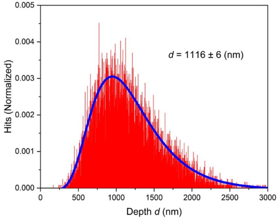
**Figure S6.** A simulation of the electron penetration depth (EDXS measurement) in BFO ceramic using the CASINO software<sup>18</sup>. The fitting curve (blue) shows a maximum at around 1  $\mu\text{m}$ . This electron penetration depth is much deeper than the penetrating depth of the implanted  $^{111\text{m}}\text{Cd}$  (12 nm) as presented in Fig. S1.
