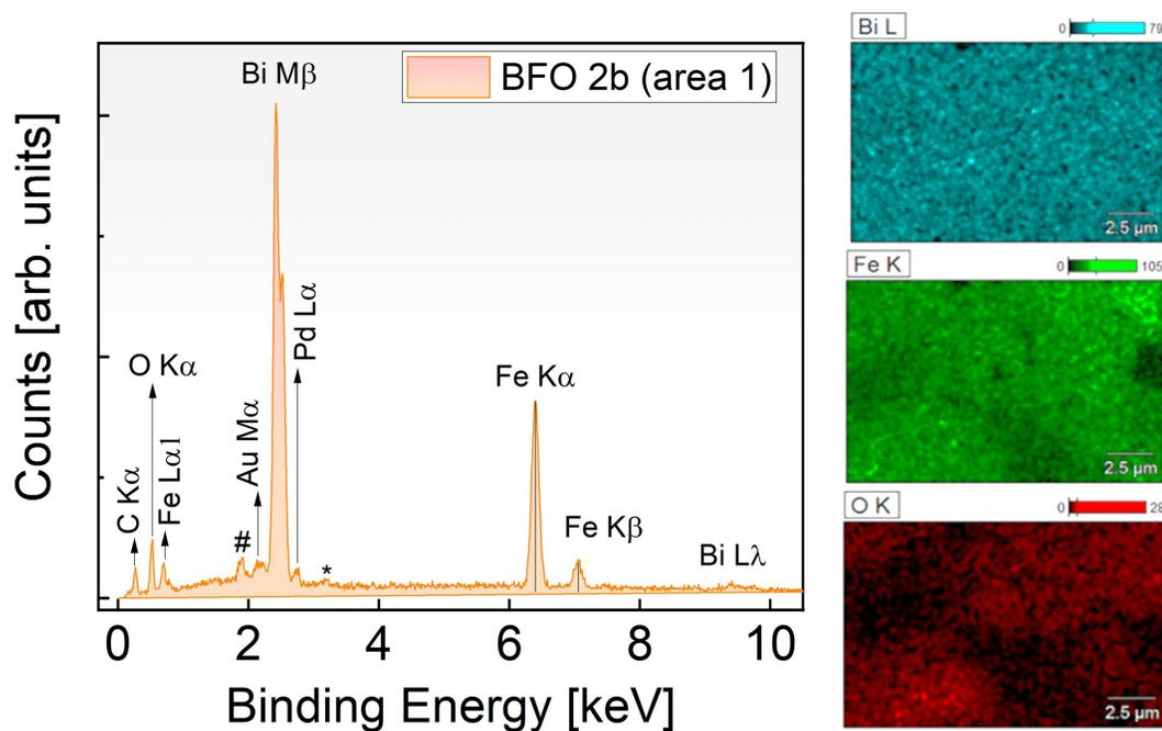
**Figure S5.** The EDXS spectra and elemental mapping of sample BFO2b. The unassigned peaks (#, \*) might have originated from the sample holder and carbon residues of the carbon tape that was used to attach the sample to the sample holder.
