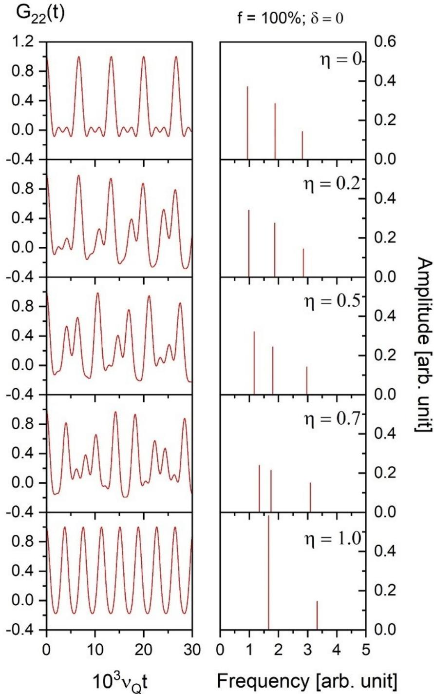
**Figure S3.** (left) Simulated perturbation factor  $G_{22}(t)$  of the static electric quadrupole interaction for any value of quadrupole interaction frequency  $v_Q$ , with one probe site ( $f = 100\%$ ), with no damping ( $\delta = 0$ ), and different asymmetry parameters  $\eta$  in the electric coordinate systems<sup>17</sup>. (right) The corresponding Fast Fourier Transforms (FFTs) of the transition frequencies.
