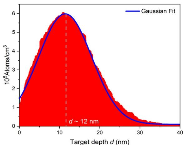
**Figure S1.** Simulation of distribution of stopping range of implanted  $^{111m}\text{Cd}$  isotope in BFO using SRIM 2008<sup>1</sup>. The Gaussian fit (blue curve) shows the mean value about 12 nm. This means that the pure beam of  $^{111m}\text{Cd}$ , with an energy of 30 keV, after hitting the BFO target at the incident angle of about  $0^\circ$ , will penetrate about 12 nm ( $d$ : penetrating depth) through the BFO target.
